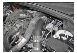
27. Install the provided coupling hose (08186) onto the mass air sensor housing, and then install the  $K\&N^{\circ}$  intake tube into the hose. Install the tube and mass air sensor assembly onto the filter adapter and into the coupler at the turbo inlet. Adjust the mass air sensor and intake tube for best fit and then secure with the provided hose clamps. **NOTE: once everything is adjusted, secure all six of the hose clamps.**
