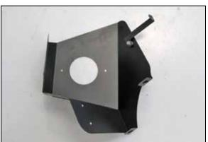
14b. On 2016 and later model vehicles, install bracket (064343) onto the heat shield as shown using the provided hardware and spacer. **NOTE: The spacer is to be placed between the**
