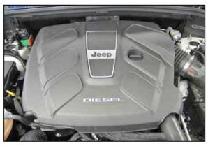
2. Lift up the decorative engine cover and remove it from the engine.
