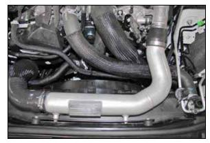
13. Install the intercooler pipe assembly and secure with the provided hose clamps and hardware, tighten the bracket mounting bolts at this time.
