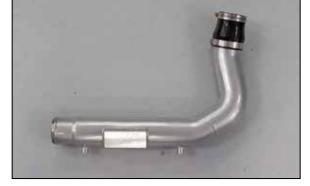
11. Install the provided step coupler (5-255) onto the K&N $^{\odot}$  intercooler pipe and secure with the provided hose clamp.
