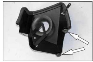
19. Install the air filter housing grommets into the heat shield as shown.
