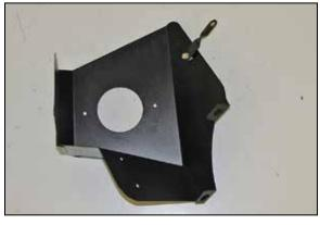
14a. On 2015 and earlier model vehicles, install bracket (070702) onto the heat shield as shown using the provided hardware and spacer. **NOTE: The spacer is to be placed between the bracket and heat shield.**
