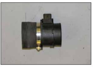
25. Install the provided coupling hose (08496) onto the air filter housing side of the mass air sensor and secure with the provided hose clamp.
