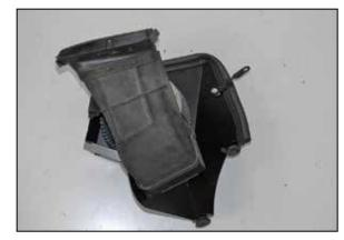
21. Install the fresh air intake scoop into the mounting bracket installed onto the heat shield assembly.
