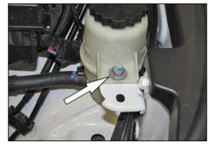
22a. On 2015 and earlier model vehicles, remove the P/S reservoir mounting bolt shown. **NOTE: This bolt will be reused in the next step.**
