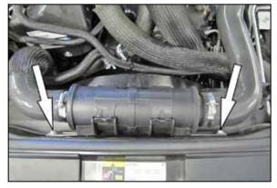
9. Loosen and remove the two bolts securing the intercooler muffler chamber to the core support then remove the muffler chamber and hose from the vehicle.
