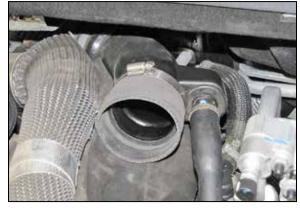
26. Install the provided coupling hose (084036) onto the turbo inlet pipe and secure with the provided hose clamp.
