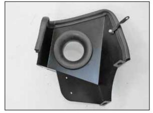
16. Install the filter adapter into the heat shield and secure with the provided hardware.
