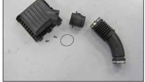
24. Remove the mass air sensor from the upper air filter housing and disconnect the intake tube. **NOTE: Remove the O-ring from the mass air sensor housing.**
