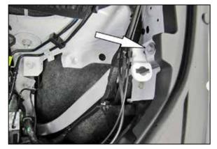
22b. On 2016 and later model vehicles, remove the fender mounting bolt shown.
