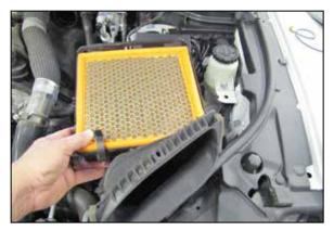
7. Lift up the lower air filter housing to dislodge it from the mounting grommets and then remove the housing from the vehicle.
