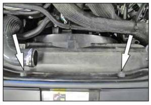
10. Install the two provided rubber mounted studs into the core support as shown. The studs will thread into the holes for the bolts which secure the muffler chamber.
