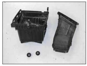
18. Remove the fresh air intake scoop and two of the mounting grommets from the lower air filter housing.
