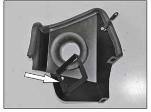
17. Install the fresh air intake scoop mounting bracket onto the heat shield and secure with the provided hardware.
