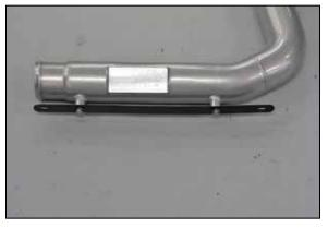
12. Install the provided bracket onto the K&N<sup>®</sup> intercooler pipe and secure with the provided hardware.
