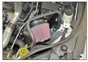
23. Install the heat shield assembly onto the air filter mounting studs and place the mounting bracket in position and the secure with the factory bolt removed in step #22.
