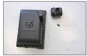
9. Remove the mass air sensor from the factory upper air filter housing.
