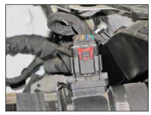
15. Reconnect the mass air sensor electrical connection.
