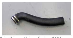
7. Install the provided coupling hose (08690) halfway onto the K&N® intake tube and secure with the provided hose clamp as shown.
