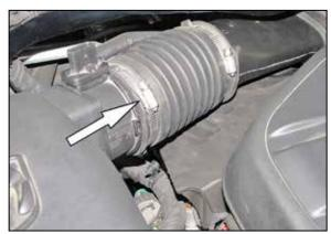
3. Loosen the hose clamp securing the factory intake tube to the mass air sensor.
