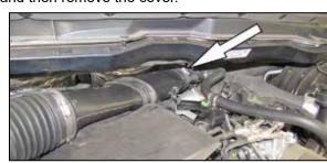
6. Loosen the hose clamp securing the intake tube to the turbo inlet hose. Lift up the intake tube to dislodge it from the mounting stud and then remove the tube from the vehicle.
