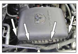
4. Release the four clips securing the upper air filter housing and then remove the housing and air filter.
