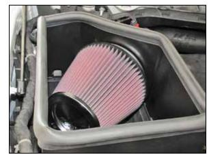
16. Install the K&N® air filter onto the filter adapter and secure with the provided hose clamp. NOTE: Drycharger® air filter wrap; part # RF-1042DK is available to purchase separately. To learn more about Drycharger® filter wraps or look up color availability please visit http://www.knfilters.com®.
