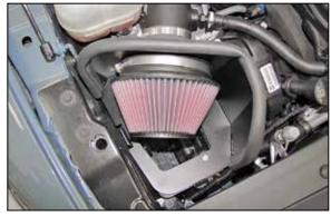
18. Install the K&N $^{\odot}$  air filter onto the filter adapter and secure with the provided hose clamp.
