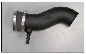
13. Install the provided quick disconnect npt fitting into the K&N<sup>®</sup> intake tube as shown. **NOTE: Plastic NPT fittings are easy to cross thread. Install the vent fitting "hand" tight, then turn it two complete turns with a wrench.**
