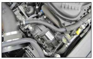
17. Install the crank case quick connect fitting into the factory crank case vent hose and connect it to the fitting installed into the  $K\&N^{\oplus}$  intake tube. **NOTE: Trim the provided hose as needed and adjust so that there are not any kinks in the hose.**  3. If road test is fine, you can now enjoy the added power and performance from your kit.
