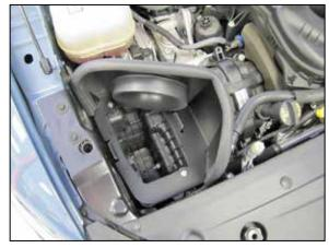
10. Install the heat shield assembly so that the mounting studs engage with the factory mounting grommets.
