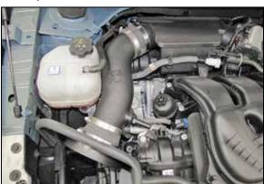
16. Install the K&N<sup>®</sup> intake tube into the coupling
