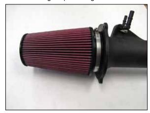
14. Install the air filter onto the end of the K&N® intake tube and secure with the provided hose clamp.
