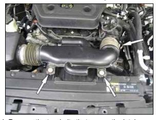
4. Remove the two bolts that secure the intake tube to the core support. Loosen the hose clamp securing the intake tube to the throttle body.
