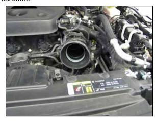
16. Install the provided step coupler onto the throttle body and secure with the provided hose
