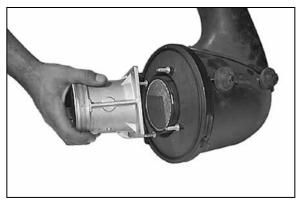
7. Remove the mass air sensor from the air cleaner.
