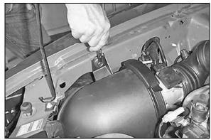
4. Loosen and remove the bolt that retains the air cleaner assembly.
