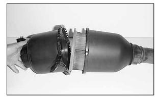
14. Disassemble the air cleaner assembly.
