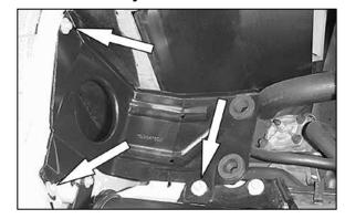
9. Loosen and remove the three bolts that retain the air cleaner mounting bracket.
