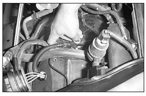
34. Reconnect the secondary mass air sensor electrical connection and reattach the wiring harness retaining clip to the inner fender apron.
