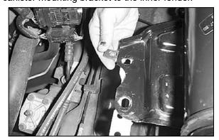
13. Remove the two clip nuts from the evaporative canister bracket lower mounting point as they will not be reused.
