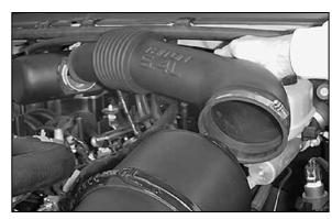
7. Remove the stock intake tube.
