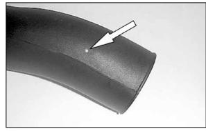
22. On models equipped with an external air temperature sensor, drill out the drill point in the K&N® intake tube using a 11/16" drill bit.
