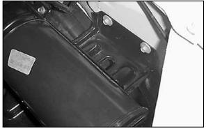
12. Loosen the two bolts that retain the evaporative canister mounting bracket to the inner fender.
