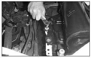
11. Loosen and remove the bolt that retains the evaporative canister mounting bracket.
