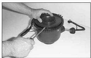
15. Using a flat blade screwdriver, push in and release the four clips that retain the mass air sensor retaining plate.
