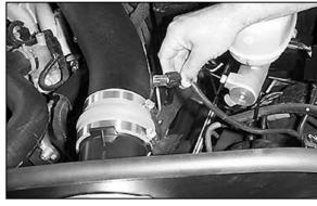
36. On models equipped with an external air temperature sensor, reconnect the air temperature sensor electrical connection and relocate the wiring harness retaining clip to front hole in the inner fender apron.
