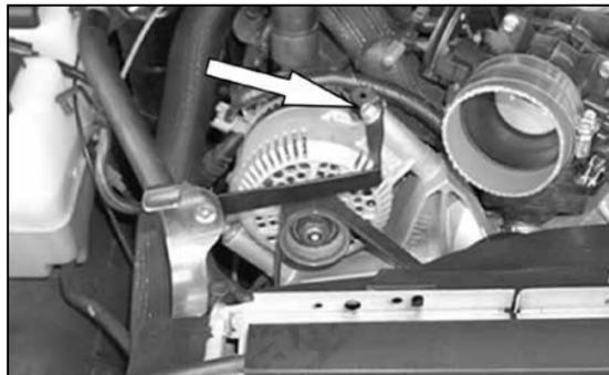
14. Remove the upper alternator bolt and harness clip, then secure the saddle bracket assembly to the alternator as shown.
