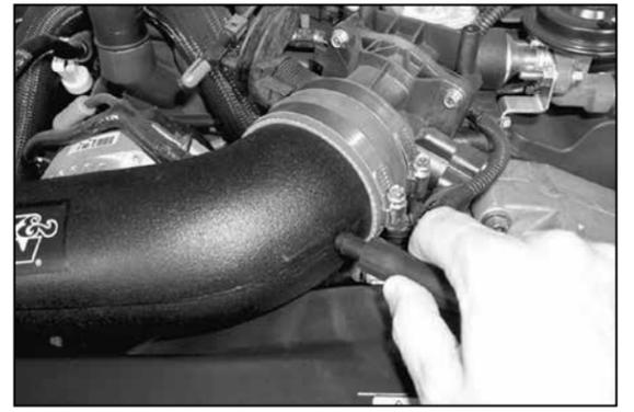
18. On vehicles that come equipped with a second vent line, line up the vent hose on the intake tube and make a mark on the intake tube for drilling.
