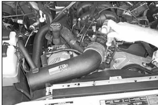
17. Install the K&N intake tube onto the throttle body and line it up with the saddle bracket assembly as shown.
