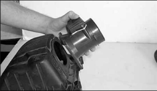
8. Loosen and remove the four bolts that secure the mass air sensor, then remove the mass air sensor as shown.
