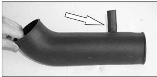
16. Install the rubber hose onto the K&N intake tube as shown.
