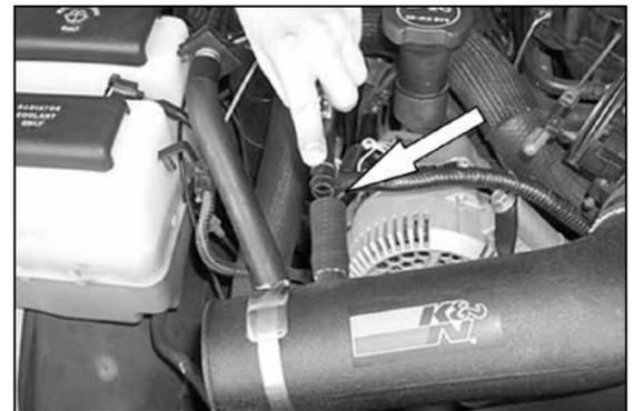
20. Re-connect the crankcase vent hose to the K&N intake tube as shown.
