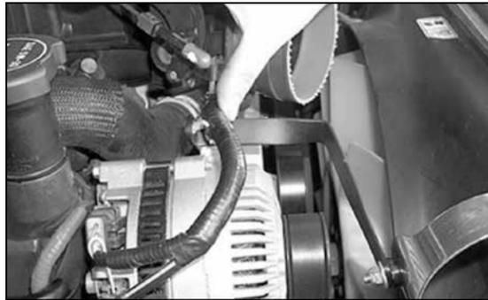
15. Push the wire harness push clip into the hole on the saddle bracket as shown.
