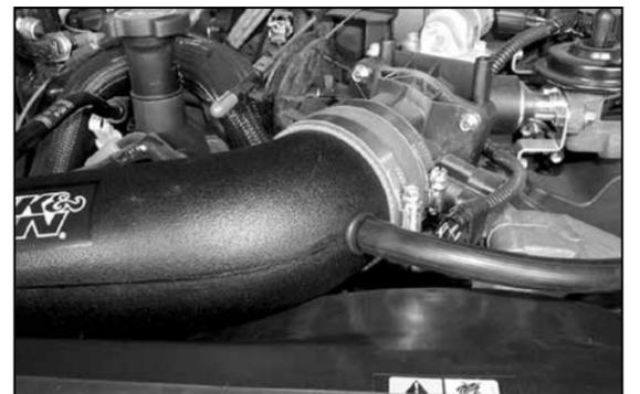
21. Vehicles that come equipped with a second vent line, reconnect as shown
