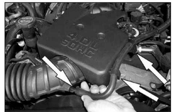
5. On vehicles that come with a second vent line, remove hose from intake tube then release the two clips that retain the hose to the engine cover.
