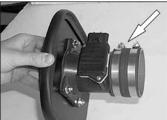
11. Assemble the silicone hose and the hose clamps onto the heat shield assembly as shown.
