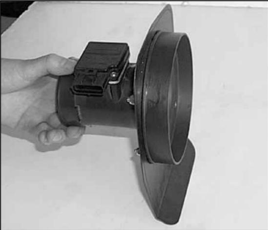
9. Assemble the mass air adapter, gaskets, heat shield and mass air sensor as shown.
