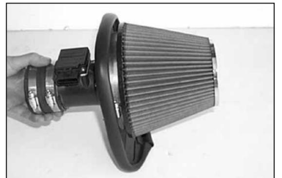
22. Assemble the K&N Air filter onto the heat shield assembly as shown.
