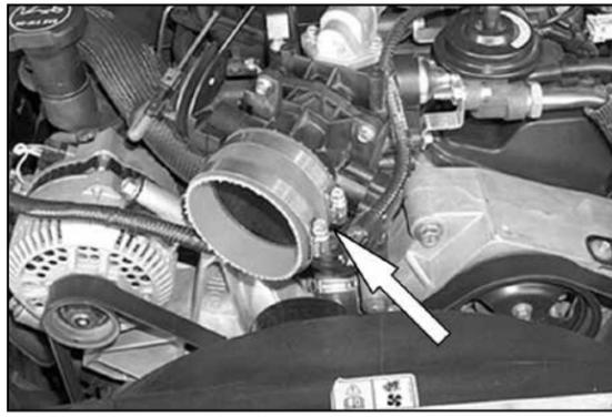
12. Install the silicone hose (08630) and the hose clamps onto the throttle body as shown.
