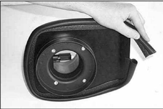
10. Apply the trim seal to the heat shield assembly as shown.
