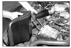
23. Slide the K&N® intake assembly into the silicone hose on the throttle body as shown.
