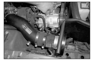
24. Line up the support bracket with the A/C compressor and secure with the original bolts removed in step 13 using a 13mm wrench.
