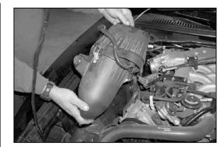
7. Pull firmly upwards to release the air cleaner from the factory grommets, then remove the air cleaner as shown.
