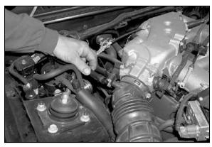
4. Disconnect the crank case vent hose from the rubber intake as shown
