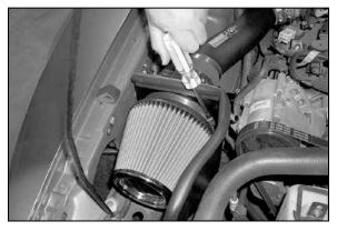
26. Install the K&N<sup>®</sup> Air filter and secure with the provided hose clamp as shown. Adjust intake tube and tighten all clamps completely.
