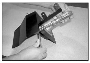
15. Using the provided hardware, assemble the support bracket onto the heat shield using a 10mm wrench as shown.
