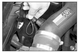
27. On 1999-2000 vehicles reconnect the air temperature sensor electrical connection.
