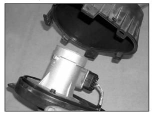
9. Using a flat blade screwdriver, depress the tabs to release the mass air sensor cover from the mass air sensor base plate as shown.
