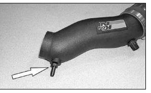
20. Install the 3/8" vent into the K&N<sup>®</sup> intake tube with a 9/16" wrench as shown. NOTE: Plastic NPT fittings are easy to cross thread. Install the vent fitting "hand" tight, then turn it two complete turns with a wrench.
