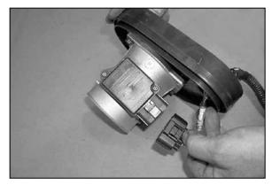
10. Disconnect the mass air sensor electrical connection from the mass air sensor as shown.
