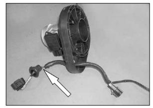
11. Remove the mass air sensor wire harness from the base plate as shown.
