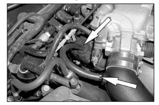
14. Using the provided hardware assemble the mass air adapter, heat shield, gaskets, and the mass air sensor as shown using a 10mm wrench or nut driver.
