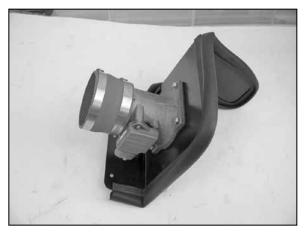
15. Install the silicone hose (08051) onto the mass air sensor with the provided hose clamps.
