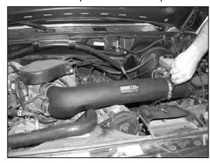
16. Install the new K&N<sup>®</sup> intake tube onto the throttle body, then secure the intake tube to the saddle bracket as shown.
