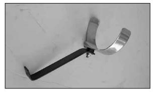
8. On vehicles that come equipped with A/C, assemble the saddle bracket onto bracket (07164) as shown.
