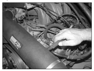
21. Reconnect the crank case vent onto the valve cover, then connect to the intake tube as shown. Trim hose for best fit.
