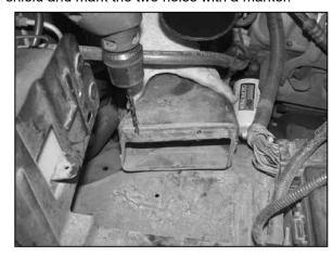
18. Remove the mass air assembly and drill two 1/4" holes were marked in the previous step.
