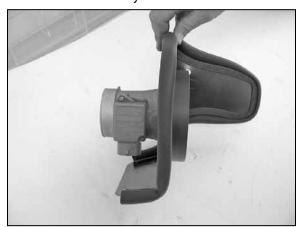
14. Assemble to mass air sensor to the heat shield and filter adaptor using the provided gaskets and hardware as shown.
