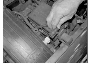
3. Disconnect the temp sensor electrical connection.
