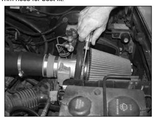
22. Install the Filtercharger to the mass air assembly as shown.
