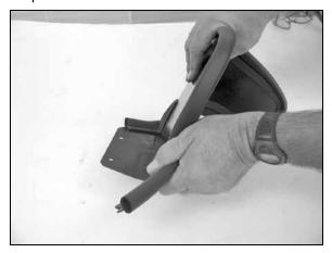
11. Install edge trim onto heat shield as shown. Trim if needed.
