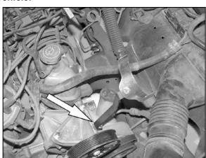
9a. On vehicles that do not come equipped with A/C, mount the saddle bracket assembly from step 8a onto the idler pully bracket as shown.
