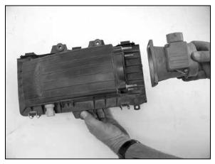
12. Remove the mass air sensor from the factory airbox as shown.
