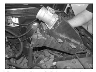
7. Remove the three bolts that secure the air box to the vehicle then remove air box from vehicle.
