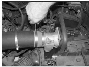
19. Reinstall the mass air assembly and secure with the provided hose clamps.
