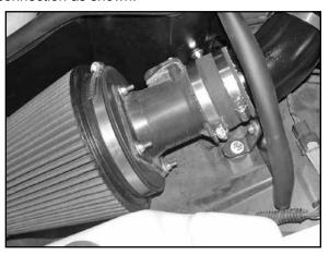
26. Install the mass air assembly onto the intake tube and adjust for best fit before tighting hose clamps.
