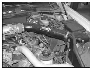
19. Install the K&N® intake onto the throttle body and line it up with saddle bracket assembly. **Note: Do not tighten completely.**
