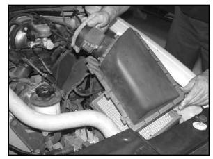
7. Release the 2 clips which reatins the airbox lid then remove the lid from the vehicle.
