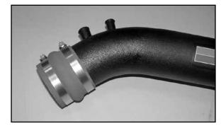
18. Install the provided silicone hump hose (087121) onto the K&N<sup>®</sup> intake tube with the provided hose clamps.
