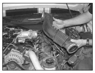
6. Loosen the hose clamp at the throttle body and at the mass air sensor then remove the stock air intake tube as shown.
