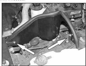
14. Install the heat shield into vehicle and attach to the two outter brackets.
