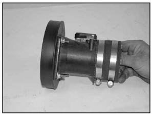
23. Install the silicone hose (08690) onto the mass air sensor with provided hose clamps as shown.
