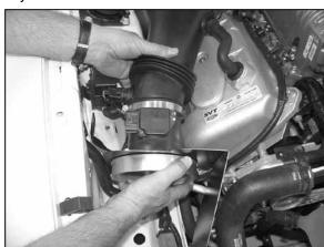
16. Install the mass air assembly onto the intake tube.
