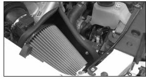
22. Reinstall the mass air assembly onto the intake tube and secure the brackets with the provided sheet metal screw and 6mm bolt onto the "L" bracket.
