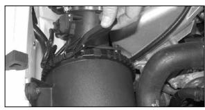
3. Release the filter clam shell clamp as shown.
