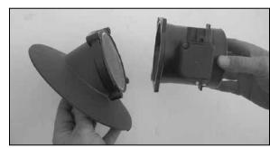
8. Remove the mass air from the air filter housing using a 10mm wrench as shown.
