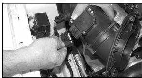
6. Disconnect the mass air electrial connection.
