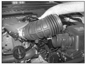
4. Remove the intake tube from vehicle. NOTE: Disconnect the three vent lines under the intake tube before removing from vehicle.
