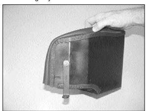
11. Install the "L" bracket onto heat shield as with the provided hardware as shown.
