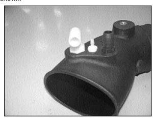
16. Install the provided vent fitting onto the new  $K\&N^{\otimes}$  intake tube as shown.
