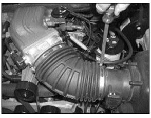
3. Loosen the hose clamp at the throttle body and mass air sensor as shown.
