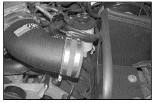
27. Install the silicone hose (08050) onto the intake tube with the provided hose clamps
