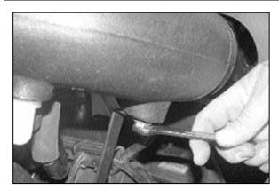
22. Connect the new intake tube to the bracket with the provided hardware as shown.
