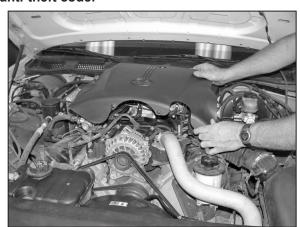
2. Loosen and remove the bolt that retains the engine cover to the engine with a 1/4 extension, then remove engine cover.
