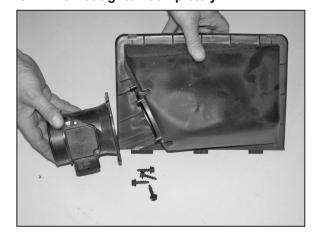
21. Remove the four bolts that retain the mass air sensor to the air box lid, then remove the mass air sensor from lid.
