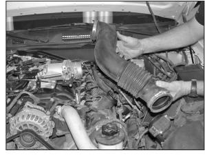
6. Loosen the hose clamp at the throttle body and at the mass air sensor then remove the stock air intake tube as shown.
