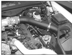
20. Install the K&N® intake onto the throttle body, then secure the tube to the saddle bracket assembly with the provided hose clamp.
