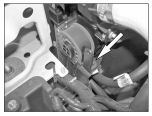
12. Using the bolt that was removed in the previous step install bracket (07879) onto the radiator support as shown.
