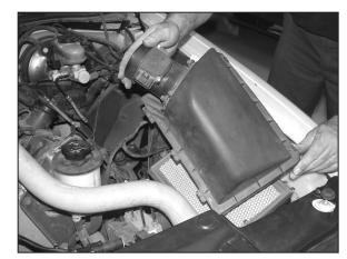
7. Release the 2 clips which retain the air box lid, then remove the lid and filter from the vehicle.
