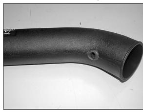
18. On vehicles that come with external temp sensor drill out the drill point with a 3/4 drill, then install the provided grommet as shown.
