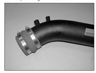
19. Install the provided silicone hump hose (087121) onto the K&N $^{\otimes}$  intake tube with the provided hose clamps.
