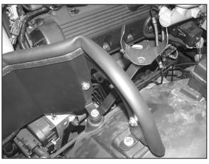
17. Install the saddle bracket assembly and the provided bracket (07093) onto the rubber mounted stud using the factory nut that was removed in step 8. onto vehicle as shown.
