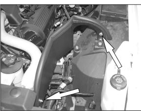
15. Install the heat shield onto the vehicle and attach to the outter brackets as shown.
