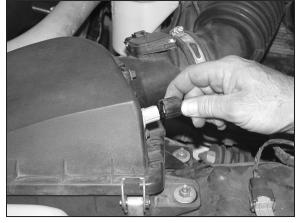
4. Disconnect the temp sensor electrical connection.
