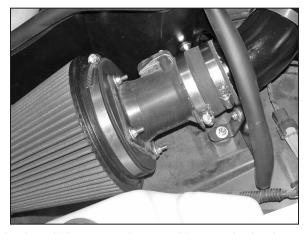
27. Install the mass air assembly onto the intake tube and adjust for best fit before tighting hose
