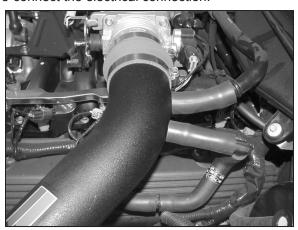
29. Reconnect the crankcase vent and idle air hose onto the new intake tube with the provided silicone hoses as shown.
