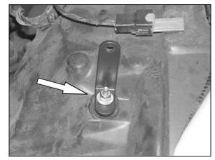
13. Install the provided bracket (07879) onto the inner wheel well as shown.
