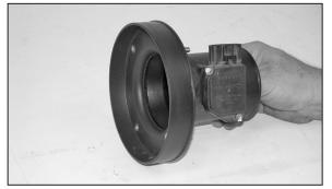
23. Assemble the filter adaptor onto the mass air sensor with the provided hardware as shown.
