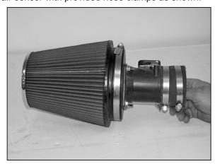
25. Install the air filter onto the mass air assembly as shown.
