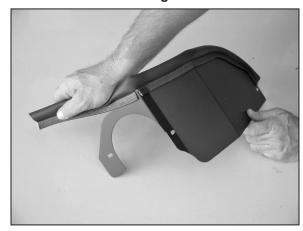
14. Install edge trim onto heat shield as shown. Trim if needed.
