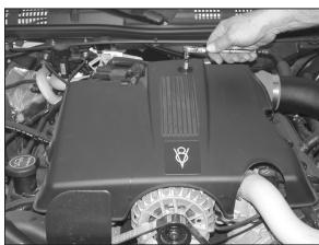
30. Re-install the engine cover that was removed in step 2.
