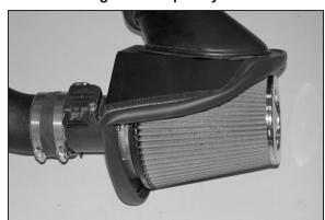
20. Attach the air filter element to the adapter using the provided hose clamp.
