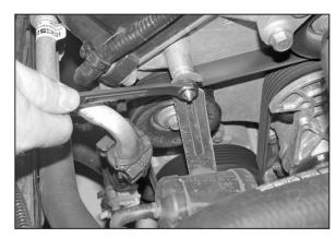
21. Loosen and remove the nut from the stud that secures the a/c line bracket on the front of engine.
