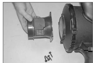
9. Loosen and remove the four bolts retaining the mass air sensor to the airbox, remove the mass air sensor.
