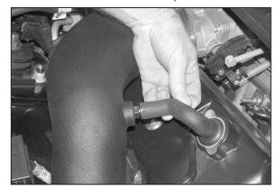
25. Install the crank case vent hose to the K&N® intake tube.
