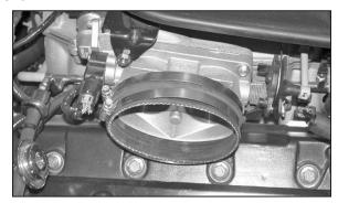
16. Attach silicone hose (08623) to the throttle body as shown.
