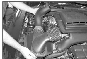
22. Install the K&N® intake assembly, by sliding the bracket onto the protruding a/c line mounting stud as shown. Reconnect the fresh air duct to the hood scoop.
