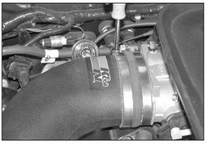
23. Secure the silicone hose to the throttle body using the hose clamp provided.
