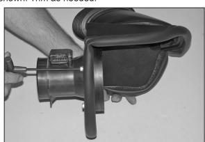
14. Assemble the mass air sensor, heat shield and adapter using the gaskets and hardware provided.
