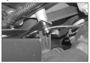
24. Secure the bracket to the a/c line mounting stud with the nut removed in step #20.
