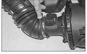
8. Loosen the hose clamp and detach the intake tube from the mass air sensor.
