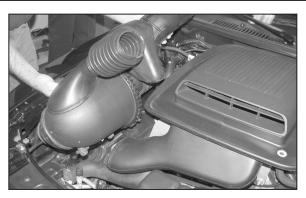
7. Remove the entire intake assembly from the vehicle.
