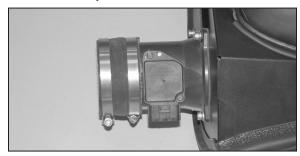
18. Attach silicone hose (08630) to the mass air sensor as shown.
