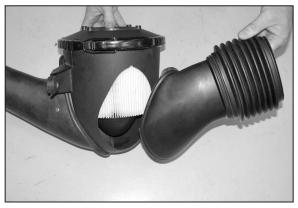
10. Separate the cold air duct from the airbox assembly.
