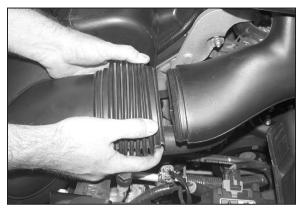
6. Separate the intake tube duct at fresh air intake inlet.
