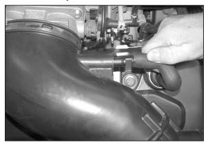
5. Detach the crank case vent hose from the intake tube.
