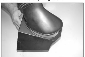
12. Snap the cold air duct removed in step 10 into the K&N® heat shield as shown.
