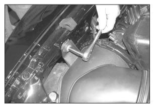
4. Loosen and remove the bolt that secures the air cleaner assembly to the inner fender.
