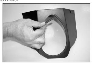
11. Install the 1/4 trim into the heat shield as shown.
