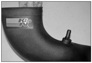
17. Install provided crank case vent fitting into K&N® intake tube as shown.
