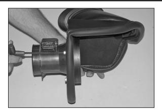
15. Attach the bracket to the mass air sensor as shown.
