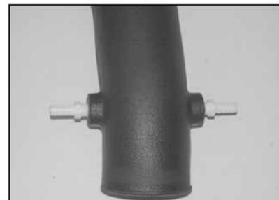
24. Install the provided NPT fittings into the intake tube as shown.
