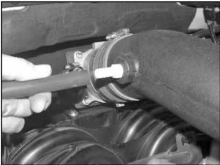
30. Install the provided silicone vent hose onto the valve cover and onto the K&N® intake tube as shown.
