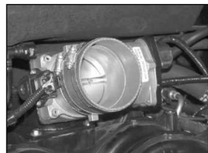
26. Install silicone hose (#08630) onto the throttle body with the provided hose clamps as shown.
