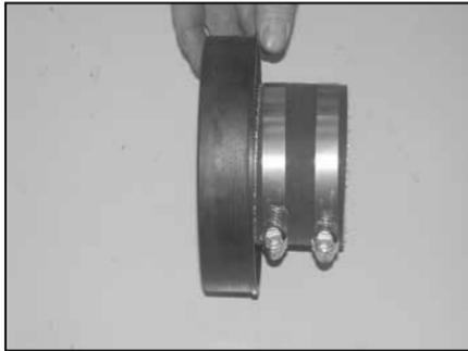
32. Install the silicone hose (#08630) onto the K&N® filter adapter and secure with the provided hose clamp as shown.
