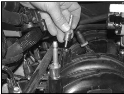
30b. Re-install the factory air box mounting studs with the provided spacers as shown.
