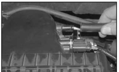
3a. On vehicles equipped, disconnect the brake booster vent line from the air filter housing as shown.
