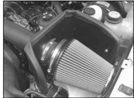
34. Install the K&N® air filter assembly onto the K&N® intake tube as shown and secure with the provided hose clamp.
