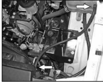
17b. Install the supplied coolant recovery hose and secure with the provided hose clamps.
