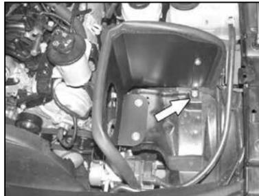
18. Install the heatshield as shown and secure with the provided hardware.
