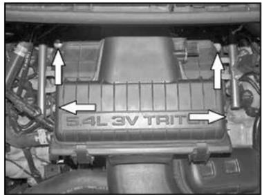
4. Remove the four air box mounting bolts shown with a 10mm socket.
