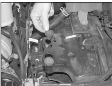
17. Install the provided nut inserts into the air box mounting holes as shown.
