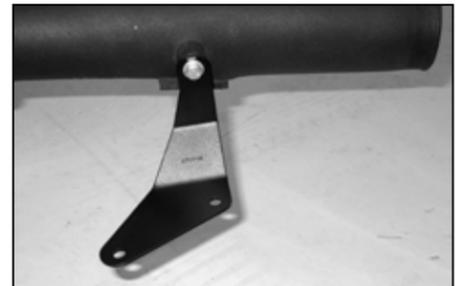
25. Install the tube mounting bracket (070118) onto the K&N® intake tube as shown with the provided hardware.
