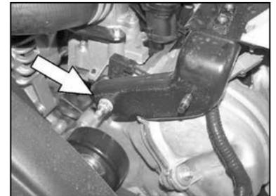
8. On vehicles that are equipped with the intake tube support bracket, reinstall one of the 13mm nuts removed in step #7 onto the lower mounting stud and tighten.
