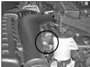
5. Remove the intake tube mounting bolt shown.
