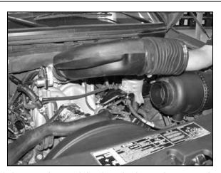
3. Loosen the stock intake tube hose clamps, and remove the intake tube from vehicle.
