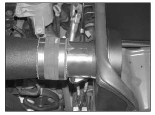
21. Install the mass air sensor assembly onto the  $K\&N^{\otimes}$  intake tube and secure with the provided hose clamp.
