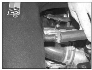
19. Install the provided silicone vent hose onto the valve cover and onto the K&N $^{\mbox{\tiny \ensuremath{\$}}}$  intake tube as shown.
