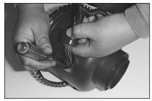
11. Slide the rubber grommet back and disconnect the primary mass air sensor electrical connection, using a flat blade screwdriver.
