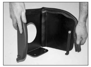
7. Install the edge trim onto the heatshield as shown. Trim if needed.
