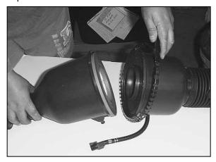
10. Open the air cleaner assembly and isolate the mass air sensor assembly.
