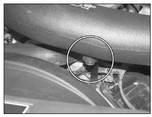
18. Attach the K&N<sup>®</sup> intake tube to the tube mounting bracket with the provided hardware.
