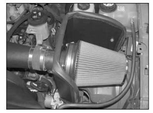
23. Install the K&N<sup>®</sup> air filter and secure with provided hose clamp.
