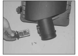
16. Remove the mass air sensor from the factory air box with the T20 "TORX" wrench provided.
