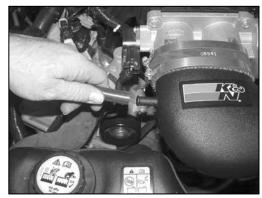
20. Install the supplied vent hose onto the vent port on the valve cover and secure with the provided hose clamp, then onto the K&N<sup>®</sup> intake tube as shown.
