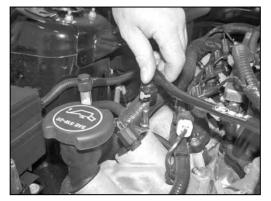
3. Rotate the green locking tab clockwise and then disconnect the crank case breather hose from the valve cover as shown.
