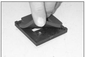
17. Install the provided gasket to the back of the  $K\&N^{\otimes}$  mass air sensor adaptor plate as shown.
