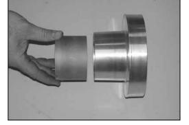
22. Vehicles that come equipped with Hydracarbon trap, place the Hydrocarbon trap into the filter adapter as shown.
