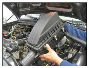
6. Pull up on the rear of the air box assembly to dislodge it from the mounting grommets and then remove the air box from the vehicle.
