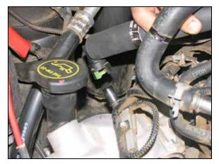
3. Rotate the green locking tab on the crank case vent connector at the valve cover counter clockwise and then pull up and disconnect the crank case vent as shown.
