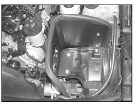
10. Install the heat shield and secure with the provided hardware as shown.
