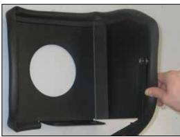
7. Install the long edge trim onto the heat shield as shown.
