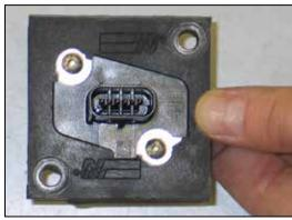
17. Install the mass air sensor into the mass air sensor adapter and secure the assembly with the provided hardware.
