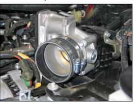
20. Install silicone hose (#08690) onto the throttle body and secure with the provided hose clamp.
