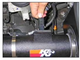
28. Re-attach the mass air sensor secondary connection to the power steering reservoir bracket, then connect the mass air sensor electrical connections as shown.
