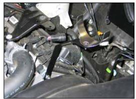
22. Install the tube mounting bracket assembly onto the stud protruding from the cylinder head. Secure with the provided hardware.
