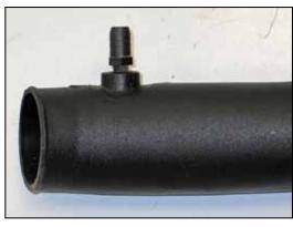
19. Install the  $\frac{1}{4}$ " NPT fitting into the K&N® intake tube as shown.
