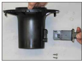
15. Remove the two mass air sensor retaining screws and remove the mass air sensor as shown.
