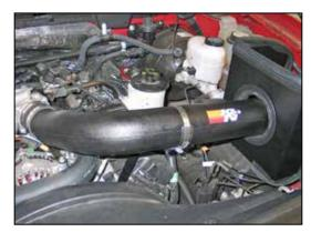
23. Install the K&N® intake tube into the silicone hose at the throttle body and align the intake tube with the saddle clamp. Secure the intake tube with the provided hose clamps.
