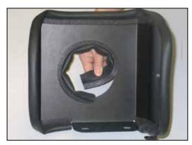
8. Install the short edge trim into the hole in the heat shield as shown.
