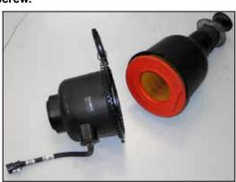
11. Release the factory air box clam shell clamp, then seperate the mass air sensor housing from the factory air box.
