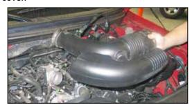
3. Loosen the stock intake tube hose clamps and remove the intake tube assembly from the vehicle.
