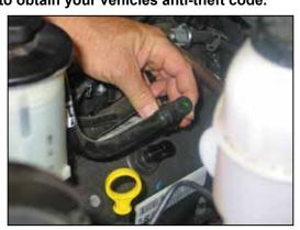
2. Rotate the crank case vent hose locking ring and disconnect the crank case vent hose from the valve cover
