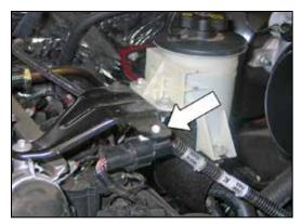
4. Un-hook the secondary mass air sensor electrical connection from the power steering reservoir bracket. Depress the electrical connection locking tabs and separate the electrical connection.
