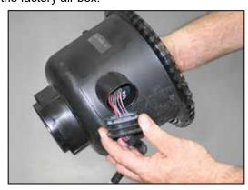
12. Slide the rubber wiring harness plug back, exposing the mass air sensor electrical connection.
