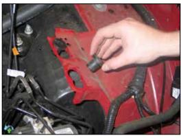
9. Remove the factory air box mounting grommets and replace them with the provided nut inserts as shown.
