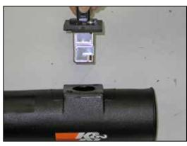
18. Install the mass air sensor assembly into the K&N® intake tube and secure with the provided hardware as shown.
