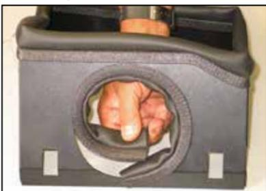
16. Install the short edge trim into the hole in the heat shield as shown.
