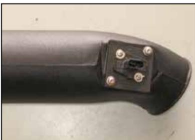
14. Secure the mass air sensor assembly onto the intake tube with the provided hardware as shown.
