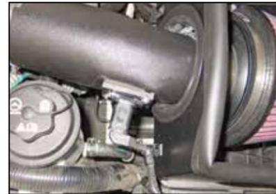
26. Re-connect the mass air sensor electrical connection as shown.
