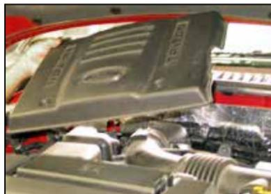
4. Remove the engine cover as shown.
