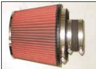
22. Install silicone hose (#08630) onto the air filter adapter and secure with the provided hose clamp.
