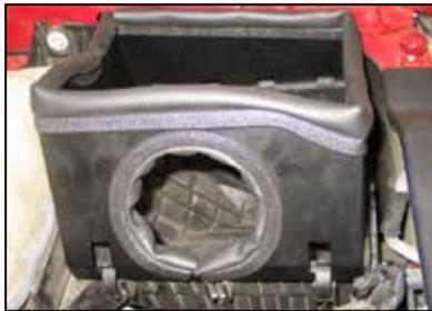
18. Install the heat shield and secure with the two remaining latches as shown.
