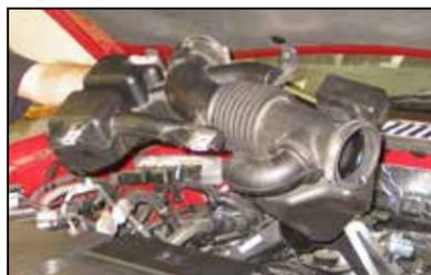
6. Remove the factory inlet tube as shown.
