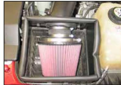
25. Secure the K&N® air filter assembly onto the K&N® intake tube with the provided hose clamp as shown.
