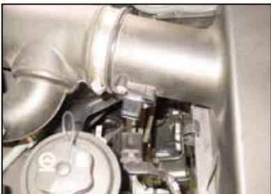
2. Release the red locking tab and disconnect the mass air sensor electrical connection.
