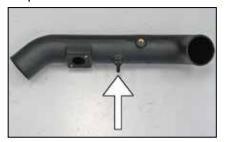
16. Install the provided 3/8" hose fitting into the K&N<sup>®</sup> intake tube as shown.
