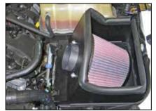
13. Install the heat shield/filter assembly onto the lower airbox and secure with the factory airbox retaining clips.
