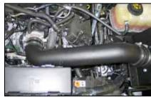
22. Install the K&N<sup>®</sup> intake tube assembly into the silicone hose at the filter adapter and then into the silicone hose on the throttle body and secure with the provided hose clamps.
