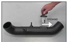
21. Install the mass air sensor assembly into the  $K\&N^{\circ}$  intake tube and secure with the provided hardware.
