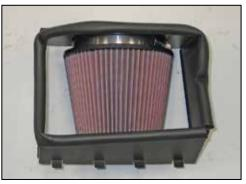
11. Install the K&N<sup>®</sup> air filter onto the filter adapter and secure with the provided hose clamp.
