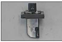
20. Install the mass air sensor into the K&N<sup>®</sup> sensor adapter as shown. Secure with the provided hardware.
