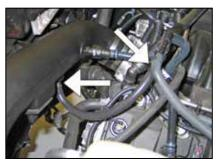
24. Install the provided silicone hose onto the 3/8" fitting installed in the K&N<sup>®</sup> intake tube and then attach the open end to the EVAP check valve.
