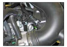
3. Rotate the locking tab and then unhook the crankcase vent hose from the factory intake tube.
