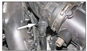
3. Disconnect the crank case vent connection.
