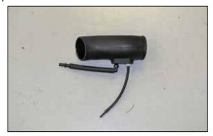
11. Install the vent hose assemblies onto the fittings installed into the K&N $^{\odot}$  intake tube.
