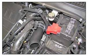
13. Install the K&N<sup>®</sup> intake tube into the coupling hose at the turbo but do not tighten at this time.
