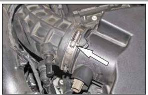
4. Loosen the hose clamp securing the intake tube to the air filter housing.
