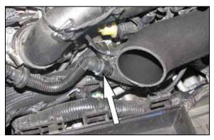
14. Connect the factory crank case vent hose to the quick connect fitting/vent hose installed into the K&N<sup>®</sup> intake tube.
