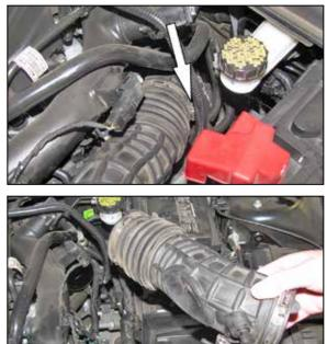
2. Disconnect the Inlet air temperature sensor electrical connection.
