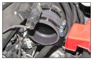
8. Install one of the hump hoses (087121) onto the turbo inlet and secure with the provided hose clamp.
