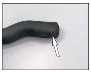
17. Install the provided grommet into the K&N<sup>®</sup> intake tube as shown.
