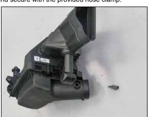
16. Remove the inlet air temperature sensor from the factory air filter housing.
