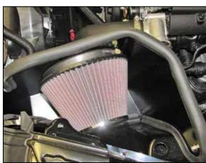
14. Install the K&N<sup>®</sup> air filter onto the filter adapter and secure with the provided hose clamp.
