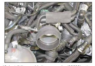
13. Install the provide hump coupler (08699) onto the throttle body and secure with the provided hose
