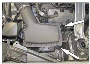
9. Release the two clips securing the air box lid and then remove the lid/intake tube assembly and the factory air filter.
