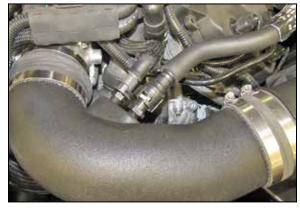
17. Connect the crank case vent and EVAP vent lines to the quick disconnect fittings installed into the K&N® intake tube as shown.
