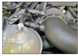
18. Connect the idle by-pass vent line to the quick disconnect fitting installed into the K&N® intake tube as shown.
