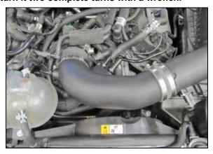
16. Install the K&N® intake tube into the hump hose at the throttle body and then into the coupling hose on the upper air box housing. Secure the hoses with the provided hose clamps
