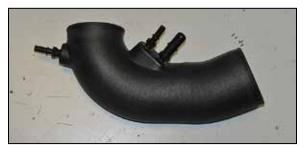
15. Install the three quick disconnect fittings into the K&N® intake tube as shown.
