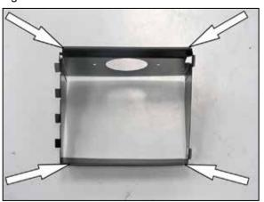
8. Install the small edge trim onto the heat shield as shown using the provided super glue to secure.
