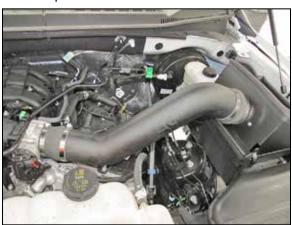
14. Install the K&N® intake tube assembly into the hose at the throttle body and onto the filter adapter, align the tube for best fit and then secure with the provided hose clamp.
