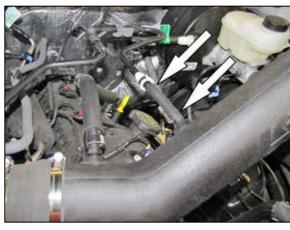
17. Install the quick disconnect union into the mating EVAP quick disconnect fitting and then connect the open EVAP vent hose to the fitting installed into the K&N® intake tube.
