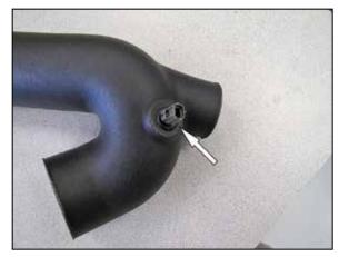
7. Remove the inlet air temperature sensor from the factory intake tube. Remove the O-Ring from the inlet air temperature sensor and then install the sensor into the K&N<sup>®</sup> intake tube using the provided grommet.
