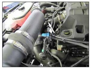
9. Using the provided extension harness, reconnect the inlet air temperature sensor electrical connection.
