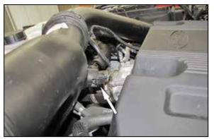
2. Disconnect the inlet air temperature sensor.
