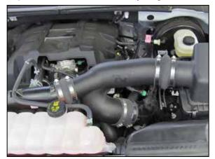
8. Install the K&N<sup>®</sup> intake tube assembly into the couplers and adjust for best fit, then secure the tube with the provided hose clamps.
