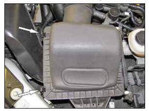
Release the two clips that secure the upper air filter housing and then remove the housing and factory air filter.
