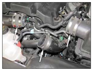
6. Install the provided coupler hoses onto the turbo inlet tubes and air filter housing and secure with the provided hose clamps.
