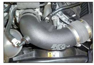
12. Install the K&N® intake tube assembly into the coupler hoses, adjust for best fit and then secure with the provided hose clamps. Connect the factory vent lines to the fittings installed into the intake tube.
