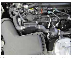
5. Remove the clamp that secures the sound tube to the sound drum and then remove the sound drum.
