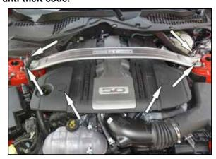
2. Remove the four nuts that secure the strut brace and then remove the strut brace from the vehicle. Using a small screw driver, pop the two nut covers off the decorative engine cover and then remove the two nuts that secure the cover to the engine , then remove the cover.
