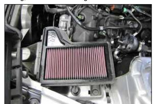
8. Install the provided K&N® air filter and then reinstall the upper housing and secure with the factory clips.
