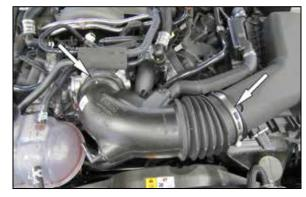
4. Loosen the hose clamps securing the factory intake tube and then remove the tube from the vehicle.
