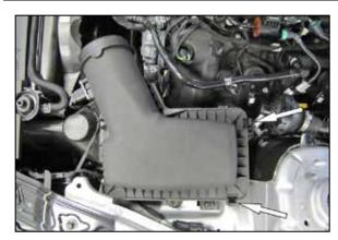
7. Release the clips that secure the upper air filter housing, remove the housing and stock air filter.
