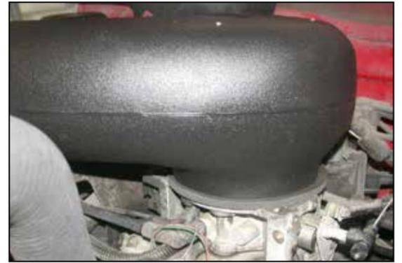
19. Install the K&N® intake tube onto the throttle body.
