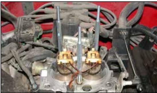
9. Install the three provided throttle body studs into the three holes from step 8.
