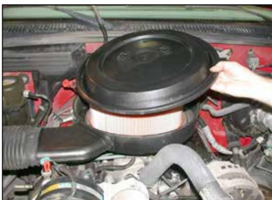
2. Loosen and remove the air cleaner wing nuts, then remove the air cleaner lid.
