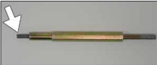
8a. Apply two drops of the provided thread locker onto the threads of the 5mm stud and then thread the stud into the tube mounting stud as shown.
