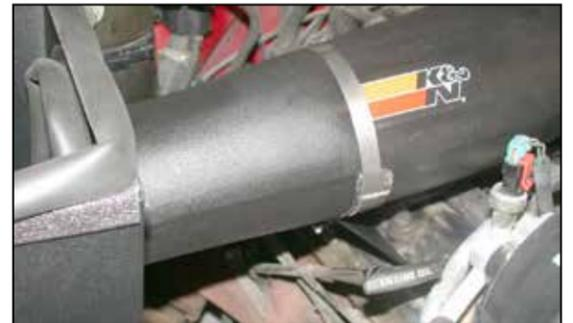
21. Secure the K&N® intake tube to the saddle bracket assembly with the provided hose clamp.
