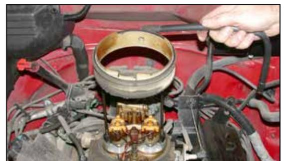
6. Remove the throttle body spacer as shown.
