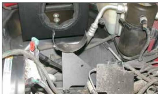
17. Install the saddle bracket assembly using the two bolts removed in step 15.
