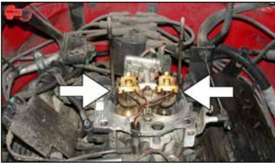
7a. On 92-95 vehicles, remove the two factory throttle body studs as shown.
