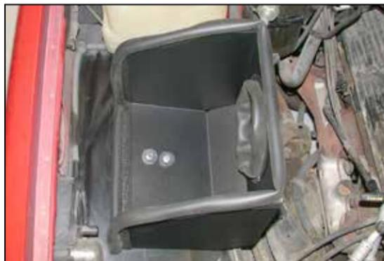
14. Install the heat shield to the inner fender using the provided hardware as shown.
