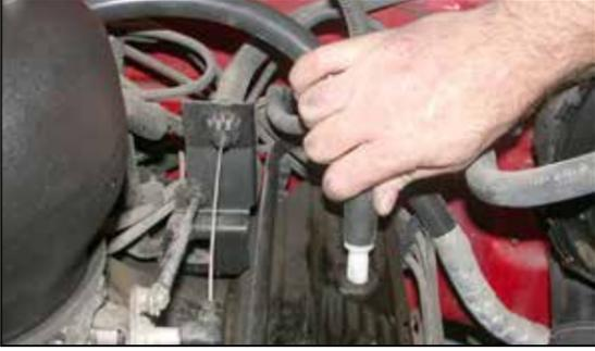
24. Install the silicone hose onto the vent on the K&N® intake tube, then push the hose mender into the grommet on the valve cover.
