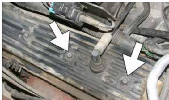
15. Remove the two valve cover bolts as shown.
