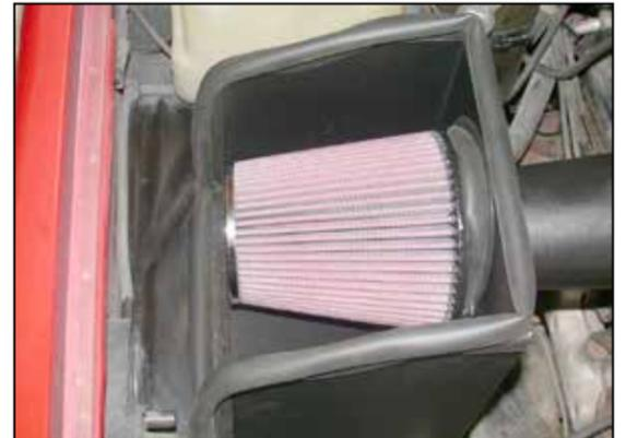
22. Install the K&N® air filter onto the K&N® intake tube as shown.
