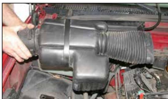
4. Loosen and remove the two bolts that secure the air inlet/resonator, then remove the assembly as shown.
