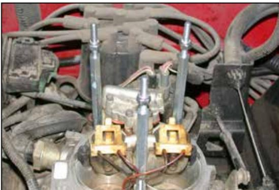
10. Install the three provided nylock nuts onto the throttle body studs approximately 3/4" down as shown.
