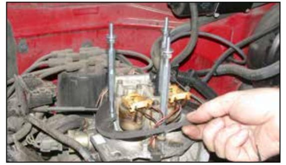
18. Remove the paper backing from the provided gasket and install the gasket onto the throttle body sticky side down.
