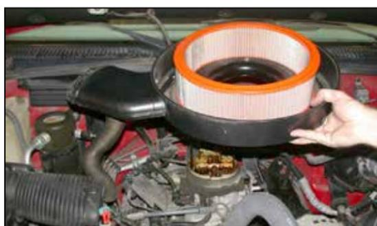
3. Disconnect the cold inlet tube and then remove the air cleaner base assembly as shown.
