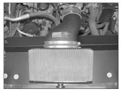
17. Install the K&N intake assembly onto the heat shield and throttle body.
