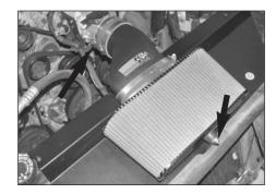
18. Align the intake tube for best clearance then tighten hose clamp at the throttle body and secure the filter to heat shield.
