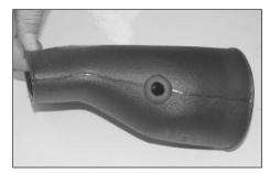
11. Install the grommet into the K&N intake tube as shown.
