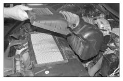
5. Remove intake from throttle body, then remove the entire upper air intake assembly.
