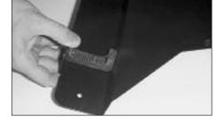
8. Install the rubber cushion onto the heat shield as shown.
