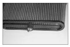
16. Install the rubber mounted stud into the threaded hole on the top plate of the filter.
