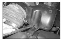
3. Pry up on the two tabs to release the clip that retains the resonator to the radiator cover.
