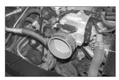
10. Install the provided silicone hose (08621) onto the throttle body with the provided hose clamps.
