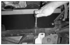
9. Secure the heat shield to the radiator core support using the bolts removed in step #6.
