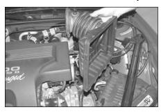
4. Release the two air box lid retaining clips, remove the air box lid and intake tube assembly as shown.
