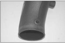
30. Install the provided grommet into the K&N intake tube as shown.
