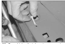
20. On vehicles that do not come equipped with a ground strap, use the 6mm self tapping bolt to thread the hole shown.
