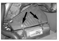
6. Loosen the two air filter housing mounting bolts shown.
