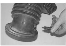
31. Remove the air temperature sensor from the factory intake tube.
