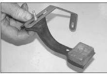
27. Place the K&N bracket (010056) behind the factory radiator bracket as shown.
