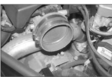
29. Install the silicone hose (08621) onto the throttle body and secure with the provided hardware as shown.
