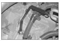
22. Install the K&N tube mounting bracket (07199) onto the stud exposed in step #21 and secure with the hardware provided.
