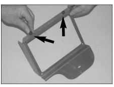
11. Install the rubber bumpers provided into the processor mounting bracket (010058) as shown.
