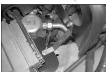
25. Install the heat shield mounting bracket (010057) using the provided hardware as shown.
