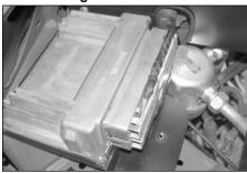
24. Reinstall the engine wiring harnesses connectors onto the engine precessor and secure with mounting bolts.
