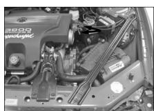
5. Remove the three body support brace mounting bolts shown, then remove the support brace from the engine compartment.
