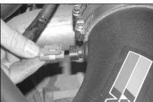
34. Reconnect the air temperature sensor electrical connection.
