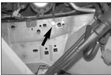
19. Remove the bolt holding the ground strap to the fender apron shown with a 10mm wrench.
