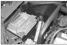
23. Set the heat shield assembly into position on the fender apron as shown.
