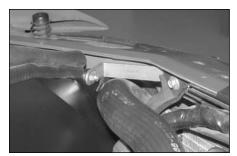
28. Reinstall the factory radiator bracket onto its original location with the K&N bracket (010056) so that the K&N bracket meets with the heat shield assembly and secure with the provided hardware.
