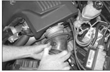
3. Pull firmly on the intake tube to separate the intake from the throttle body.
