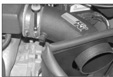
33. Install the K&N intake tube onto the throttle body, securing with the hose clamp provided, then secure the tube to the mounting bracket installed in step #22 with the provided 8mm bolt.
