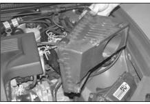
7. Tilt the air filter housing in, then lift to remove the filter housing from the mounting tabs.
