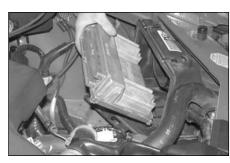
9. Remove the engine processor from its housing as shown.
