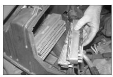
8. Loosen the center retaining bolts on the engine processor electrical connection and unplug the connectors from the engine processor.
