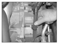
18. Remove the wiring harness retaining clip from stud protruding from the transmission case as shown.
