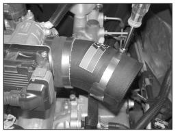
28. Install the K&N® intake tube onto the throttle body and saddle clamp as shown then secure with the provided hose clamps.
