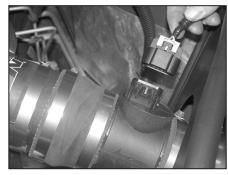
39. Reconnect the mass air sensor electrical connection.
