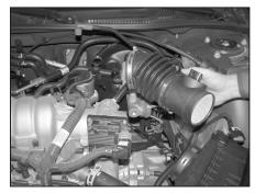
6. Loosen the hose clamps, which secure the stock intake tube to the throttle body and the mass air sensor to the stock airbox. Remove the intake tube assembly from the vehicle as shown.
