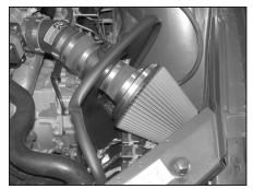
36. Install the air filter assembly onto the mass air sensor and secure with the provided hose clamp as shown.
