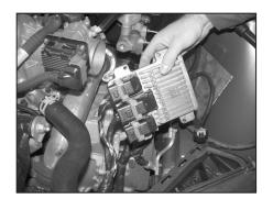
10. Unlock the engine processor from its mounting tabs and lift it out from the processor housing.
