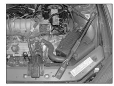
7. Remove the three body support brace mounting bolts shown, then remove the support brace from the engine compartment.
