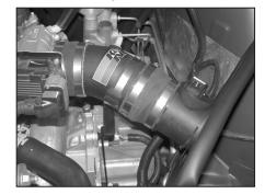
31. Install the mass air assembly onto the K&N® intake tube and secure with the provided hose clamp as shown.
