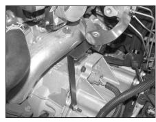
19. Install the saddle clamp assembly onto the stud exposed in step #18 and secure with the provided hardware.
