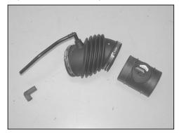
29. Loosen the hose clamp, which secures the mass air sensor to the stock intake tube, and then remove the mass air sensor and vent hose elbow from the stock intake tube.
