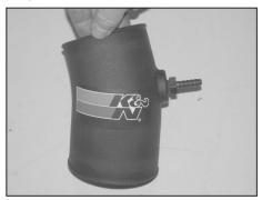
27. Install the provided NPT into the K&N $^{\ensuremath{\mathbb{R}}}$  intake tube as shown.
