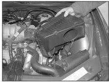
9. Tilt the air filter housing in, then lift to remove the filter housing from the mounting tabs.
