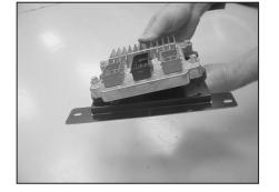
15. Install the processor with rubber mounted studs to the mounting plate with the provided 6mm nuts as shown.
