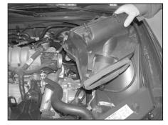
12. Pull firmly up on the engine processor housing to release it from the mounting tabs, then remove the housing from the vehicle.
