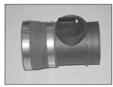
30. Install the silicone hose (08051) onto the mass air sensor and secure with the provided hose clamp as shown.
