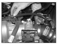
33. Install the vent hose assembly onto the NPT in the K&N<sup>®</sup> intake tube and then reconnect the elbow to the intake tube as shown.
