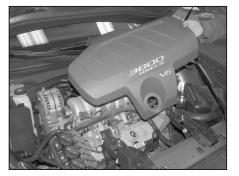
3. Lift the engine cover to remove it from the engine.
