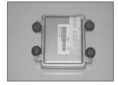
14. Install the rubber mounted studs to the processor with the provided hardware as shown.
