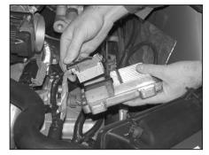
11. Unlock the engine processor electrical connections and then disconnect the connections from the processor.
