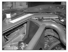
24. Remove the radiator mounting bolt shown.
