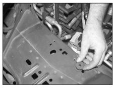
21. Install the provided inserted nuts into the airbox mounting grommet holes exposed in step #20.
