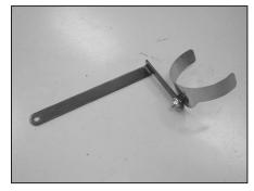
17. Install the saddle clamp onto the tube mounting bracket (010093) with the provided hardware as shown.
