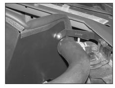
25. Install the K&N<sup>®</sup> bracket (010056) onto the heat shield and radiator mount as shown. NOTE: Use the bolt removed in step 24 and washer provided between the K&N bracket and factory bracket.
