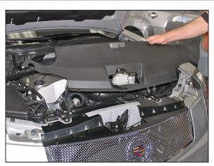
3. Dislodge the cover from the hold on clamps on the under side of the cover and then remove the cover as shown
