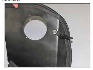
11. Install the heat shield mounting bracket onto the heat shield as shown with the provided hardware.
