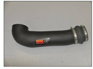
18. Install the silicone hump hose onto the K&N<sup>®</sup> intake tube as shown and secure with the provided hose clamp.
