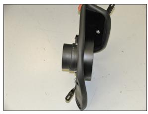
13. Install the mass air sensor onto the heat shield using the gaskets and filter adapter as shown.
