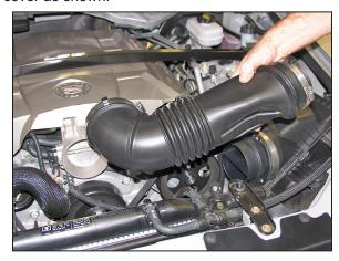
4. Loosen the two hose clamps which secure the intake tube to the throttle body and mass air sensor, then remove the intake tube as shown.
