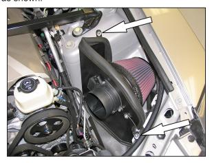
15. Install the heat shield and air filter assembly into the vehicle and secure with the provided hardware as shown.
