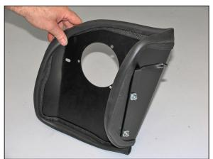
10. Install the heat shield mounting bracket onto the heat shield as shown with the provided bardware
