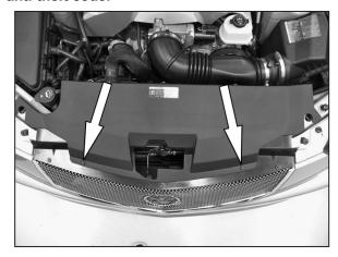
2. Release the two locking pins shown which secure the radiator cover to the radiator core support.
