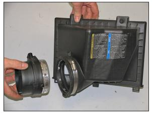
12. Loosen the hose clamp which secure the mass air sensor to the air box and then remove the mass air sensor from the air box as shown.
