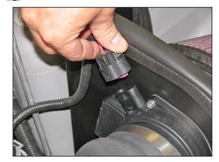
21. Reconnect the mass air sensor electrical connection as shown.
