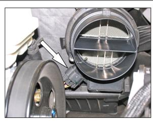
5. Disconnect the mass air sensor electrical connection shown.
