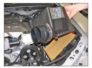
7. Lift and remove the air box lid and mass air sensor from the lower air box as shown.
