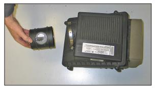
8. Loosen the hose clamp that secures the mass air sensor to the air box and then remove the mass air sensor as shown.
