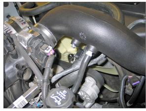
21. Clip the upper radiator hose mount into the bracket install on the K&N® intake tube.
