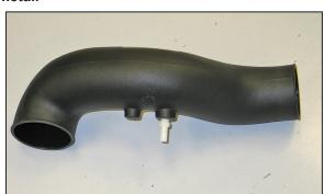
13. Install the  $\frac{1}{4}$ "npt fitting into the K&N® intake tube as shown.
