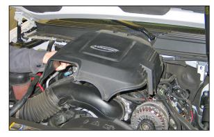
3. Pull up firmly on the engine cover to dislodge it from the mounting grommets and then remove the engine cover from the vehicle as shown.
