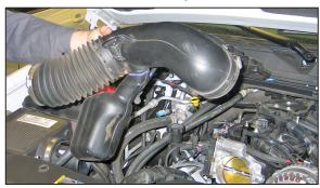
5. Unhook the upper radiator hose clip from the intake tube. Disconnect the crank case vent hose from the valve cover and then remove the intake hose from the vehicle.
