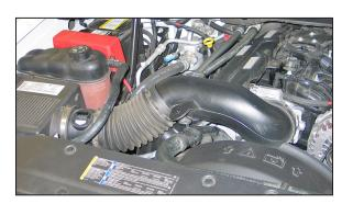
4. Loosen the two hose clamps that secure the intake tube to the throttle body and air box.
