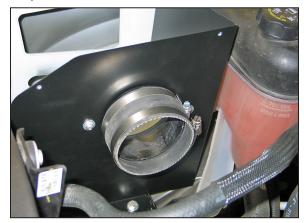
17. Install the provided silicone hose (08618) onto the filter adapter as shown and secure with the provided hose clamp.
