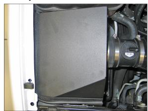
24. Install the heat shield lid onto the heat shield and secure with the provided hardware.
