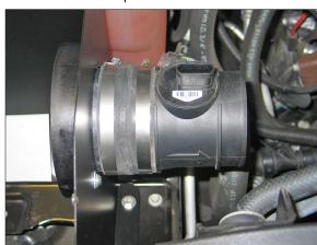
18. Install the mass air sensor into the silicone hose at the filter adapter and secure with the provided hose clamp.
