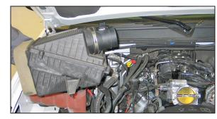
6. Pull up firmly on the air box assembly to dislodge it from the mounting grommets and then remove the air box from the vehicle.
