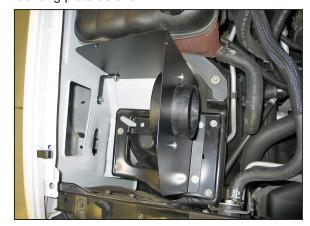
12. Install the heat shield assembly onto the air box mounting plate and secure to the inserted nuts with the hardware provided. Secure the heat shield mounting bracket to the inner fender with the hardware provided.
