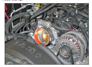
16. Install the supplied silicone hose (08625) onto the throttle body and secure with the provided hose clamp.
