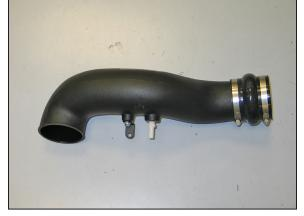
15. Install the silicone hump hose (08176) onto the  $K\&N^{\otimes}$  intake tube and secure with the provided hose clamp.
