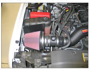
22. Install the K&N® air filter to the air filter adapter and secure with the supplied hose clamp.
