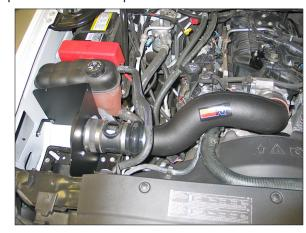
19. Install the K&N® intake tube assembly into the silicone hose at the throttle body and onto the mass air sensor as shown and secure with the provided hose clamps.
