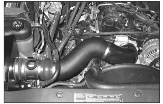
21. Install the K&N® intake tube into the throttle body and mass air sensor silicone hoses. Secure with the provided hose clamps.
