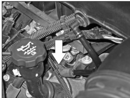
4. Disconnect the crank case vent hose from the valve cover vent port.
