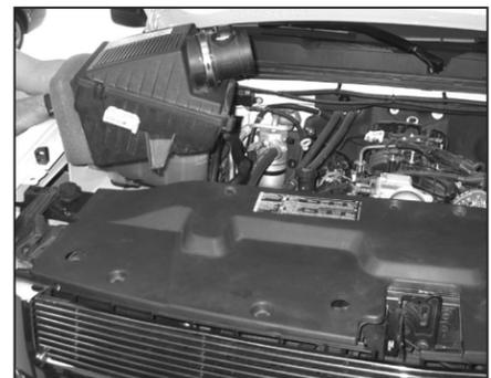
8. Firmly lift up the air box assembly to dislodge it from the mounting grommets. Then remove the air box assembly from the vehicle.
