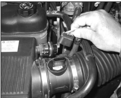
3. Disconnect the mass air sensor electrical connection.
