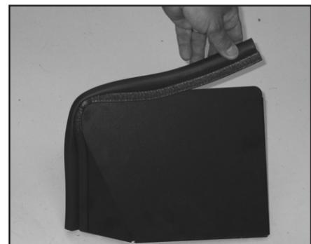
24. Install the edge trim onto the air box lid as shown.
