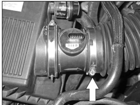
5. Loosen the hose clamp that secures the stock intake tube to the mass air sensor.
