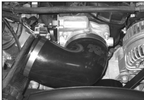
19. Install the 90° silicone hose (084053) onto the throttle body and secure with the provided hose clamp.
