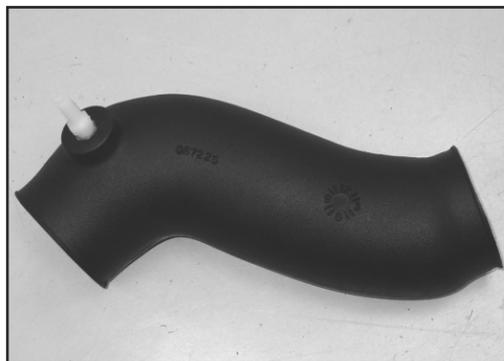
20. Install the 1/4"npt fitting into the K&N® intake tube as shown.
