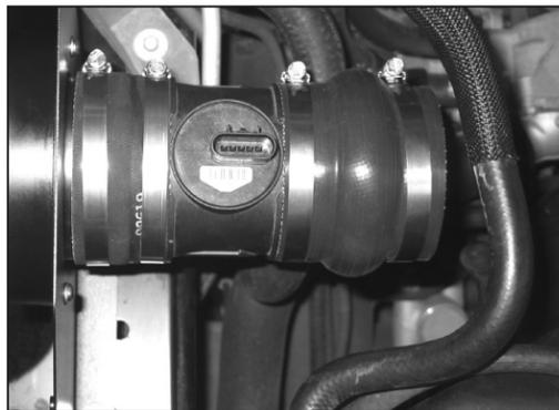
18. Install the silicone hump hose (084056) onto the mass air sensor and secure with the provided hose clamp.
