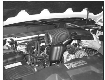
7. Unhook the stock intake tube from the mounting grommet and the upper radiator hose. Then remove the stock intake tube from the vehicle as shown.
