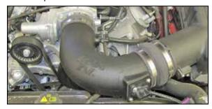
17. Install K&N® intake tube into the hose at the throttle body and then into the hose at the air filter cover, adjust the tube for proper fit and then secure with the provided hose clamps.
