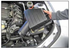
6. Release the two clips securing the air filter cover and then remove the air filter cover.
