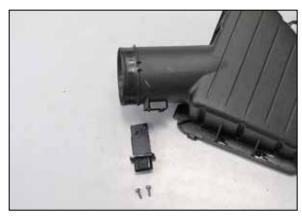
7. Remove the mass air sensor from the air filter
