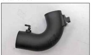
12. Install the 90° vent fitting into the K&N® intake tube as shown.
