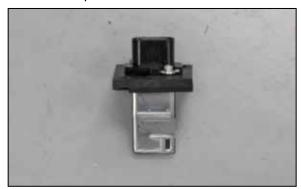
10. Install the mass air sensor into the adapter and secure with the provided hardware.
