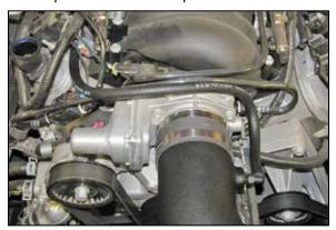
18. Connect the provided crank case vent hose to the fitting in the K&N® intake tube and then onto the valve cover port.
