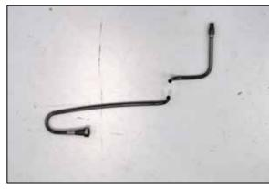
18a. On 2014 and later vehicles, it will be necessary to cut the crank case vent tube as shown. Then connect the Cut section of tube to the oil filler cap. Attach the supplied hose to the to the trimmed section of crank case vent tube.
