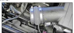
16. Install the provided coupling hose (08418) onto the air filter cover and secure with the provided hose clamp.
