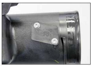
8. Using the factory screws from the previous step, install the mass air sensor block off plate and gasket.
