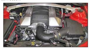
20. Reinstall the engine cover, Reconnect the negative battery cable. Double check to make sure everything is tight and properly positioned before starting the vehicle.
