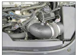
12. Install the K&N<sup>®</sup> intake tube into the hump
