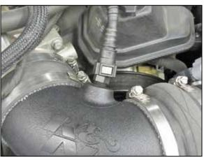
13. Connect the crank case vent hose to the quick disconnect fitting.
