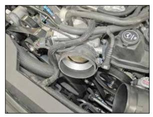
9. Install the provided coupler hose (08761) onto the throttle body and secure with the provided hose clamp.
