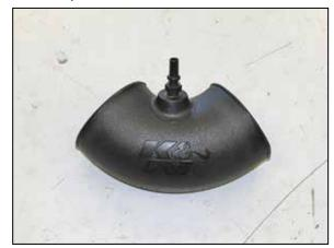
11. Install the provided quick disconnect fitting into the K&N intake tube as shown.
