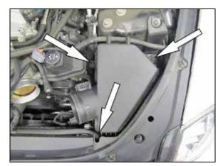
7. Loosen the three screws securing the upper air filter housing and then remove the housing and factory air filter.
