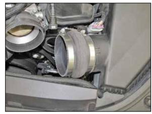
10. Install the provided hump coupler (08418) onto the air filter housing and secure with the provided hose clamp.
