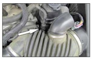
4. Release the locking tab and disconnect the crank case vent hose.
