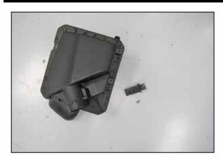
7. Remove the mass air sensor from the factory air box.
