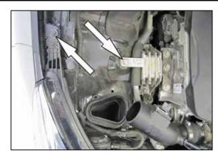
17. Remove bolts from inner fender and motor mount
