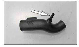
5. Install the provided 1/4" NPT quick disconnect fitting onto the  $K\&N^{\otimes}$  intake tube.
