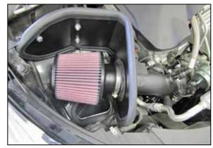
21. Install  $K\&N^{\otimes}$  air filter secure with provided hose clamp.
