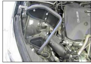
18. Install heat shield into vehicle inserting K&N® intake tube assembly through heat shield opening. Using provided hardware secure bracket (070772) to inner fender. Secure remaining bracket onto motor mount reusing motor mount bolt removed from an earlier step. Align intake tube with heat shield and tighten provided hose clamp.
