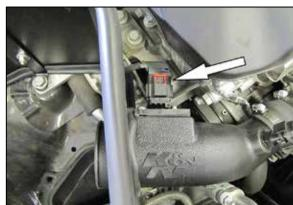
20. Reconnect mass air sensor electrical connector onto mass air sensor.
