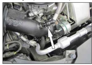
19. Connect crankcase vent line onto quick connect fitting on K&N® intake tube.
