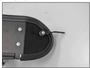
16. Install bracket assembly onto heat shield assembly with provided hardware.
