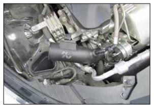
10. Install the provided coupling hose (084018) onto the turbo and secure with provided hose clamp and then Install K&N® intake tube assembly into the coupler at turbo and secure with provided hose clamp. Do not completely tighten hose clamp at this time
