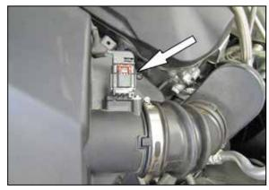
2. Disconnect mass air sensor electrical connector.
