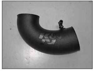
13. Install the provided 90° quick disconnect fitting into the K&N® intake tube as shown.
