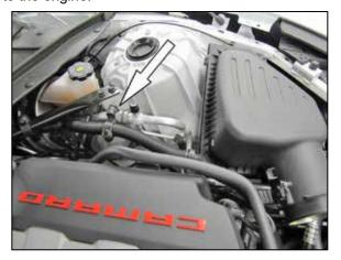
6. Disconnect the clamps securing the sound tube then disconnect the front sound tube from the rear tube and the union.
