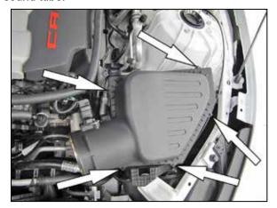
9. Loosen the five screws securing the upper air filter housing and then remove the factory air filter.
