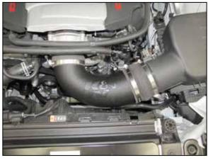
14. Install the K&N® intake tube into the hump coupler and then into the coupler at the throttle body, adjust the tube for best fit and then secure with the provided hose clamps.
