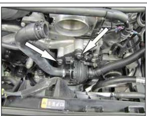
5. Remove the two bolts securing the sound drum to the engine.
