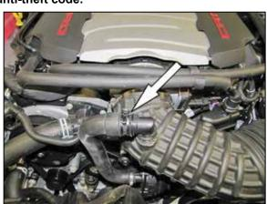
2. Release the spring clamp and then disconnect the sound tube from the intake tube.
