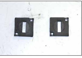
14. Install the two provided gaskets onto the  $K\&N^{\otimes}$  mass air sensor adapters.
