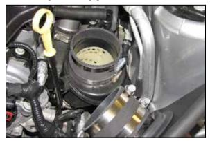
13. Install the coupling hose (08186) onto the driver's side turbo inlet and install the two coupling hoses (08711) onto the air filter. Secure the couplers with the provided hose clamps.
