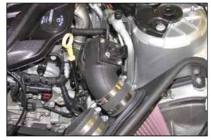
18. Install the driver's side intake tube into the coupler at the turbo and then into the coupler on the filter. Secure the tube with the provided hose clamps.
