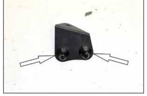
23. Install the two mounting studs onto the mounting bracket using the provided hardware.
