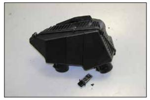
19. Remove the passenger side mass air sensor from the factory air filter housing.
