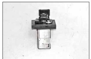
20. Install the passenger side mass air sensor into one of the K&N $^{\odot}$  adapters and secure with the provided hardware.
