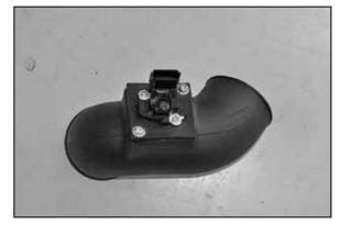
17. Install the driver's side sensor into the driver's side  $K\&N^{\otimes}$  intake tube as shown. NOTE: The opening in the sensor is to be towards the filter end of the intake tube.
