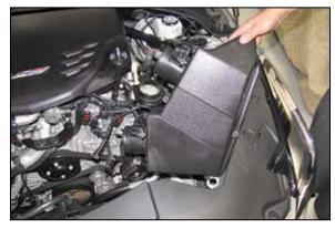
6. Lift the air filter housing assembly to dislodge it from the mounting grommets and then remove it from the vehicle.
