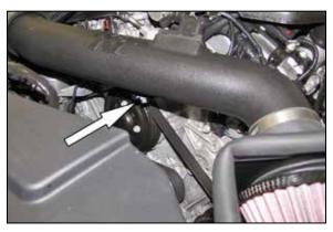
27. Connect the crank case vent hose to the quick disconnect fitting installed into the passenger side  $K\&N^{\mbox{\ensuremath{\$}}}$  intake tube.
