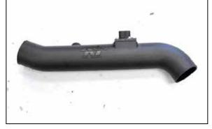
21. Install the passenger side sensor into the driver's side  $K\&N^{\textcircled{o}}$  intake tube as shown. NOTE: The opening in the sensor is to be towards the filter end of the intake tube.
