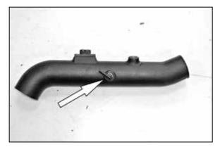
22. Install the provided quick disconnect fitting into the passenger side intake tube as shown.
