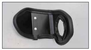
7. Install the edge trim into the hole and around the heat shield as shown.
