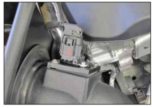
19. Reconnect the mass air sensor electrical connection.
