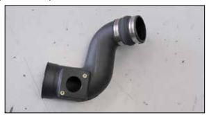
10. Install the provided hump coupler (084018) hose onto the K&N $^{\circ}$  intake tube and secure with the provided hose clamp.
