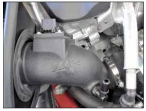
16. Install the K&N<sup>®</sup> intake tube assembly through the opening in the heat shield and then onto the Turbo inlet. Adjust the tube and heat shield for best fit and then secure them with the hose clamp and hardware.
