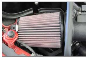
17. Install the air filter onto the K&N<sup>®</sup> intake tube and secure with the provided hose clamp. Adjust the tube and heat shield for best fit and then secure them with the hose clamp and hardware. NOTE: Drycharger<sup>®</sup> air filter wrap; part # RC-4630DK is available to purchase separately. To learn more about Drycharger<sup>®</sup> filter wraps or look up color availability please visit http://www.knfilters.com<sup>®</sup>.
