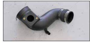
11. Install the 90° NPT vent fitting into the K&N $^{\otimes}$  intake tube as shown.
