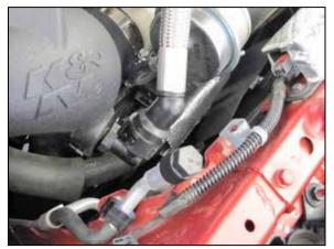
18. Connect the crank case vent hose to the fitting installed into the K&N $^{\odot}$  intake tube.
