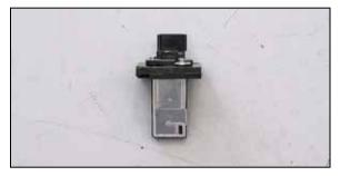
14. Install the mass air sensor into the K&N<sup>®</sup> mass air sensor adapter and secure with the provided hardware.
