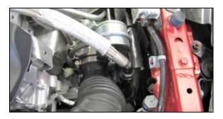
3. Disconnect the crank case vent hose. NOTE: On 2017 and later vehicles, it will be necessary to use the special tool provided (088027) to disconnect the crank case vent line. Snap the tool onto the vent tube and then slide it upwards until it unlocks the retaining clips and then disconnect the crank case vent line.
