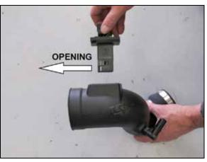
15. Install the mass air sensor assembly into the  $K\&N^{\circ}$  intake tube so that the opening in the sensor is towards the air filter end of the intake tube.
