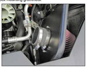
11. Install the provided coupler hose (08711) onto the filter adapter and secure with the provided hose
