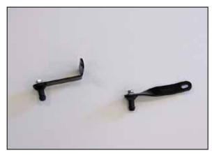
7. Install the two provided mounting studs onto the mounting brackets and secure with the provided hardware.
