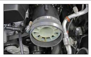
12. Install the provided coupler hose (08540) onto the turbo inlet chamber and secure with the provided hose clamp.
