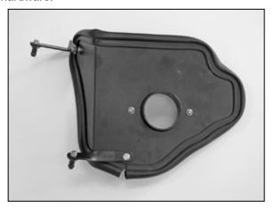
8. Install the mounting bracket assemblies onto the heat shield as shown and secure with the provided hardware.
