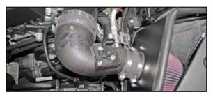
18. Install the K&N® intake tube into the hose at the filter adapter and then into the hose at the turbo chamber, adjust the tube for best fit and then secure with the provided hose clamps.
