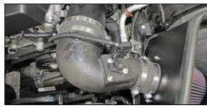
19. Reconnect the mass air sensor electrical connection and secure the wiring harness to the insert in the K&N® intake tube.
