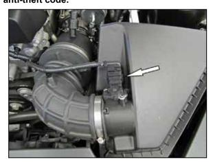
2. Release the locking tab and then disconnect the mass air sensor electrical connection and unhook the wiring harness from the intake tube.
