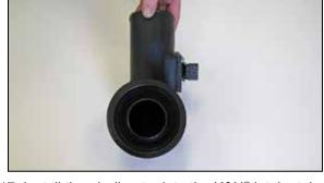
17. Install the air diverter into the K&N® intake tube so that the radius face is inside the intake tube.
