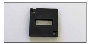
13. Install the provided gasket onto the mass air sensor adapter.
