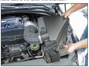
4. Lift the complete factory intake assembly up to dislodge it from the mounting grommets and then remove it from the vehicle.
