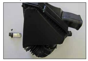
14. Remove the mass air sensor from the factory air filter housing.
