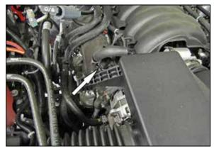
2. Disconnect the crank case quick connect vent line from the valve cover.
