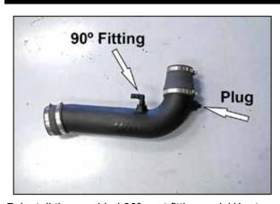
7. Install the provided 90° vent fitting and 1/4npt plug into the K&N® intake tube as shown. **NOTE: Plastic NPT fittings are easy to cross** thread. Install the vent fitting "hand" tight, then turn it two complete turns with a wrench.
