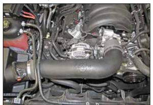
8. Install the intake tube assembly onto the air filter housing and then onto the throttle body, adjust the tube for best fit and then secure with the provided hose clamps.
