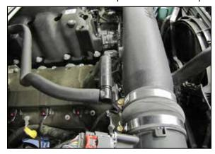
12. Using the provided hose, connect the vent hose to 90° fitting installed into the K&N® intake tube.
