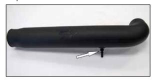
9. Install the provided quick connect fitting into the K&N® intake tube as shown.
