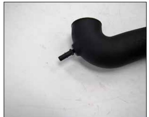
5. Install the provided quick disconnect fitting into the K&N® intake tube as shown.
