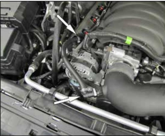
9. Install the crank case vent assembly onto the valve cover port and the fitting installed into the K&N® intake tube as shown.
