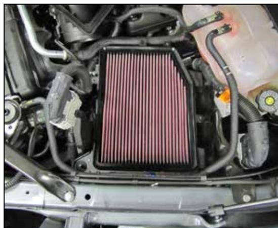
4. Loosen the three bolts that secure the upper air filter housing and then lift off the housing and replace the factory air filter with the K&N® air filter. Reinstall the upper housing and secure with the factory bolts.
