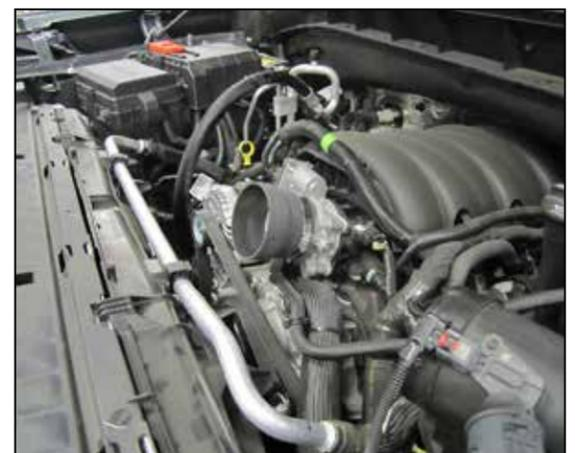
6. Install the appropriate coupler onto the throttle body and secure with the provided hose clamp. 5.3L engines will use coupler #08497, 6.2L engines will use coupler #084107.
