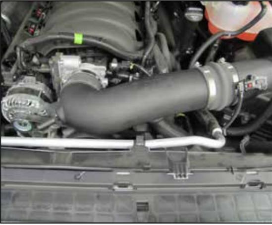
7. Install the K&N® intake tube into the coupler at the filter housing and then into the coupler at the throttle body, adjust the tube for best fit and then secure with the provided hose clamps.
