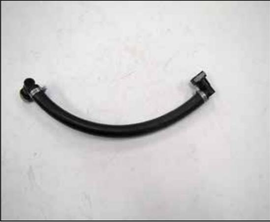
8. Assemble the crank case vent assembly as shown using the provided components.
