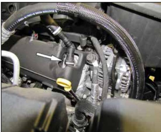
2. Disconnect the crank case vent line from the valve cover.
