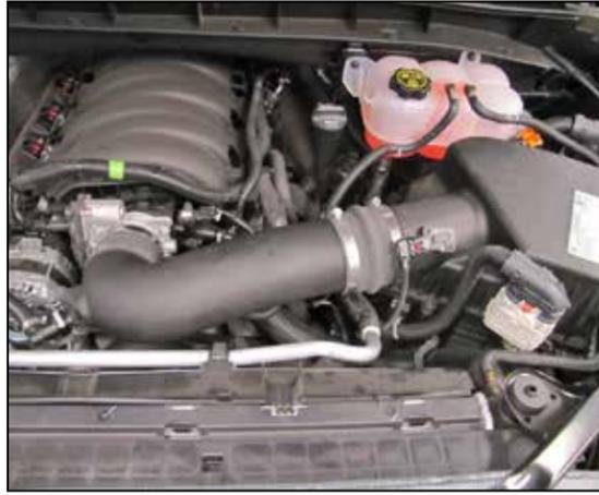
10. Reconnect the mass air sensor electrical connection.
