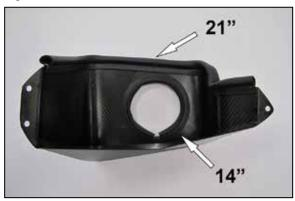
12. Install the edge trim onto the K&N<sup>®</sup> heat shield as shown.
