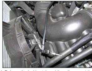
4. Release the locking tab and then disconnect the crank case vent line from the factory intake tube.
