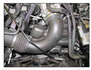
5. Loosen the two hose clamps that secure the factory intake tube and then remove the intake tube from the vehicle.
