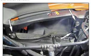
10. Install the three rubber mounted studs into the air filter housing mounting location as shown.
