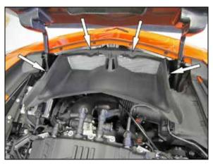
3. Loosen the four bolts that secure the air extractor duct to the radiator and then remove the extractor from the vehicle.
