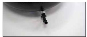
17. Install the provided crank case quick connect fitting into the K&N® intake tube as shown.
