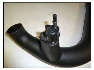
15. Remove the CCV solenoid from the factory intake tube and install it into the K&N<sup>®</sup> intake tube using the factory bolt.
