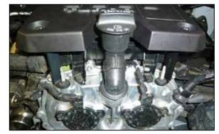
9. Install the engine cover onto the engine and secure the brackets to the factory mounting studs using the factory nuts.
