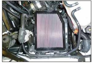
11. Install the K&N<sup>®</sup> air filter and then reinstall the upper housing and secure with the factory screws.
