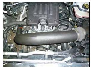
16. Install the intake tube assembly into the coupler at the air filter housing and then into the coupler at the turbo inlet, adjust the tube for best fit and then secure with the provided hose clamps.
