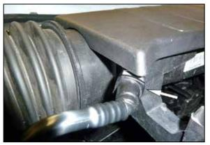
3. Depress the locking tab and then disconnect the CCV pipe from the plenum.
