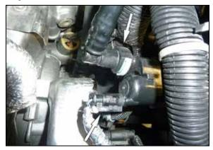
18. Connect the CCV tube to the solenoid and connect the electrical connection.
