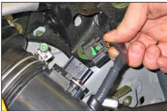
2. Depress the locking tab and disconnect the mass air sensor electrical connection. Next separate the mass air sensor wire harness from the clips, which attach to the air box.
