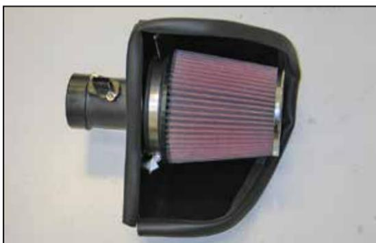
20. Install the Air Filter onto the radius filter adapter as shown.
