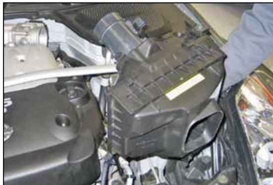
6. Lift up on the air box to dislodge it from the mounting grommet and then remove the air box from the vehicle as shown.
