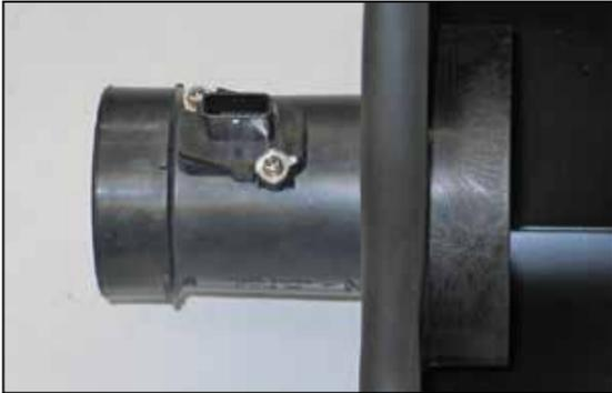
12. Reinstall the mass air sensor into the mass air sensor housing with the factory screws removed in step #9.
