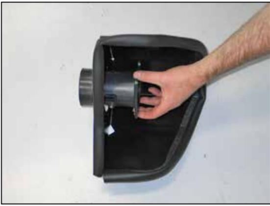
10. Pass the mass air sensor housing through the heat shield as shown.
