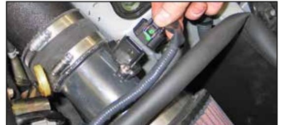
22. Reconnect the mass air sensor electrical connection and secure the wiring harness to the heat shield in the hole provided.
