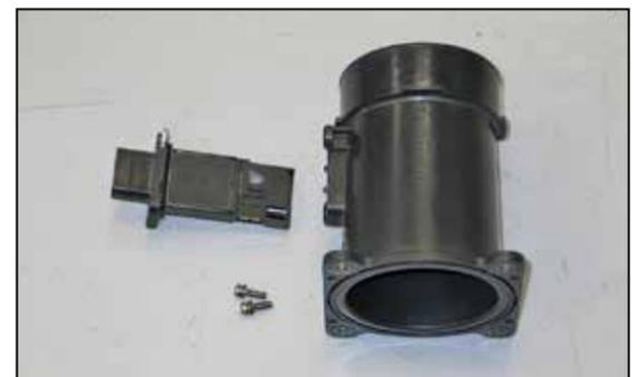
9. Remove the two screws, which secure the mass air sensor into the mass air housing, then remove the mass air sensor from the housing.
