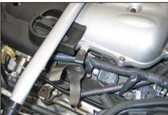
14. Install the saddle bracket assembly onto the engine using the bolt removed in step #3 as shown.
