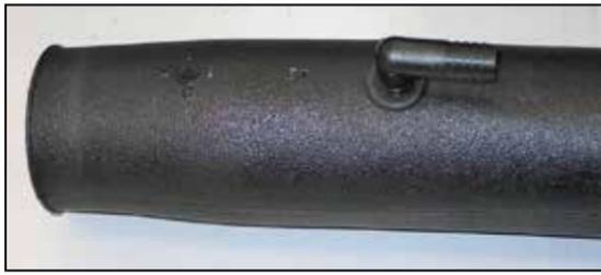
16. Install the provided 90 deg. fitting into the grommet that was installed onto the K&N® intake tube in step #15.
