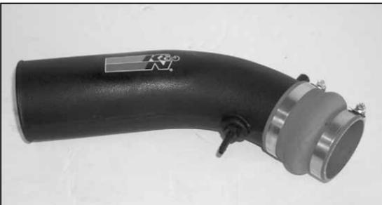
13. Install the 1/4" npt fitting onto the K&N® intake tube as shown.
