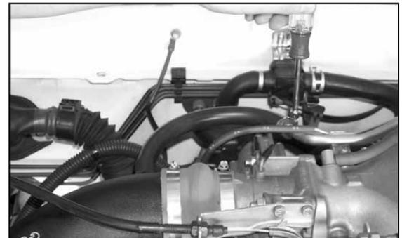
21. Remove the stock crankcase vent hose and replace it with the provided silicone hose and hose clamp. Secure it to the vent on the K&N® intake tube.
