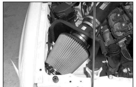
23. Install the K&N® air filter onto the filter adapter and slide the vent hose through the hole in the heat shield.
