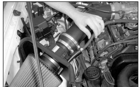
24. On vehicles equipped with a EVAP vent line attached to the airbox, connect the factory EVAP line to the hose mender/vent line installed into the K&N® air filter during step #22.
