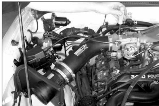
17. Slide the K&N® intake tube into the mass air adapter, then secure the other end onto the throttle body as shown.
