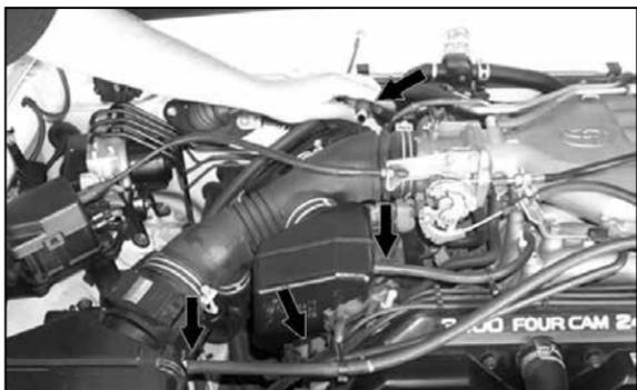
3. Disconnect the four vent hoses as shown above.
