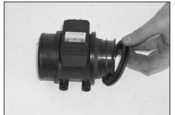
7. Remove the factory lip seal from the mass air sensor as shown.
