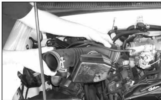
4. Unhook the wire harness from the factory intake tube, then loosen the hose clamps on the intake tube. Remove the factory intake tube as shown.
