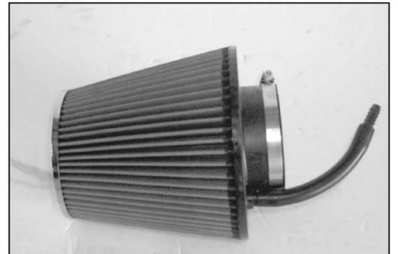
22. Install the vent hose with hose menders from step #19 into the K&N® air filter as shown.
