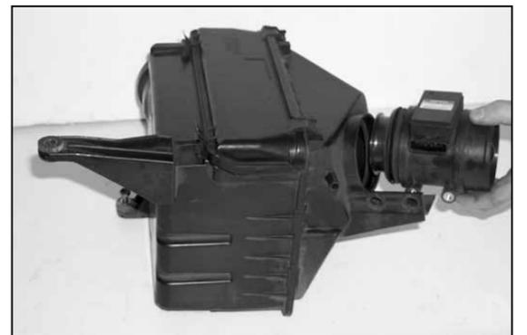
6. Loosen and remove the two bolts that secure the mass air sensor to the airbox, then remove the mass air sensor as shown.
