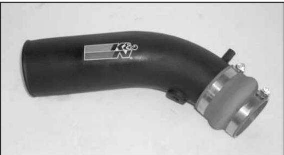
12. Install the silicone hump hose and hose clamps onto the K&N® intake tube as shown.
