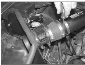
29. Install the mass air sensor onto the new K&N® intake tube as shown.
