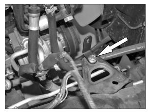
13. Mount the provided bracket (070712) onto the air box mounting tab with the provided hardware.
