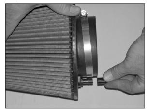
26. On vehicles that use the vacuum "T", cut two barbs off the provided hose mender. Then install the hose mender into the filter. Cut the cap plug in half, then install the plug onto the hose mender as shown.
