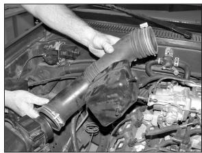
4. Loosen the hose clamps at the throttle body and air box, then remove intake tube as shown.
