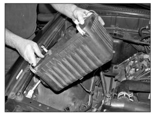
6. Remove the air box from vehicle as shown.
