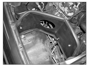
17. Using the provided hardware secure the heat shiled onto the vehicle as shown. Do not tighten completly.
