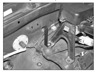
14. Remove the bolt that secures the cruise control bracket to the vehicle, then bolt the provided bracket (070952) to vehicle with the bolt that was removed.
