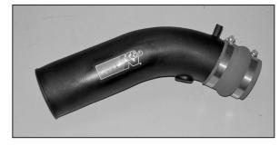
18. Install the silicone hose (08421) onto the new  $K\&N^{\odot}$  intake tube with the provided hose clamps.
