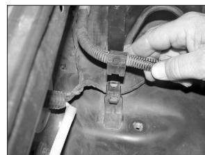
16. Disconnect the wire harness from vehicle, then locate harness on other side of bracket.
