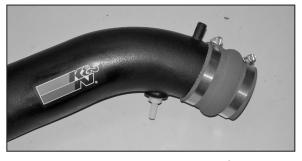
19. Install the NPT fitting onto the K&N $^{\! \rm 8}$  intake tube as shown.
