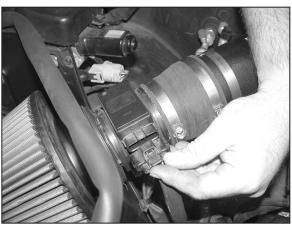
31. Reconnect the mass air sensor electrical connection as shown.
