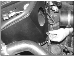
28. Reconnect the mass air sensor wiring harness onto the heat shield as shown.
