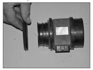
8. Remove the factory lip seal from the mass air sensor as shown.
