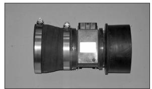
27. Install the filter adaptor onto the mass air sensor as shown.
