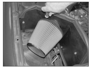
30. Install the K&N® air filter onto the filter adaptor as shown.
