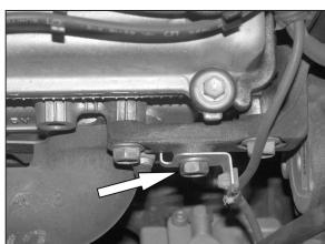
10. Loosen and remove the bolt that secures the wire harness bracket located directly behind the power steering reservoir.
