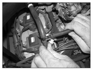
25. Install the rubber hose and vacuum "T" as shown
