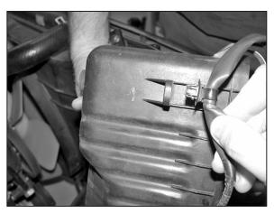
5. Remove the air box lid and filter, then remove the three bolts that secure ths air box to vehicle. Then lift the air box to release the wiring harness as shown.
